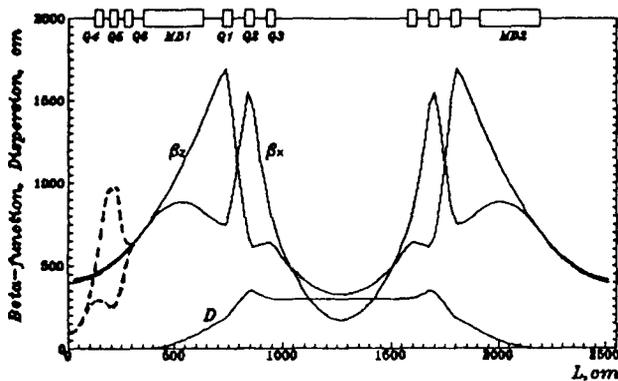
Fig.2. Beta-functions and dispersions on one-quarter of SR:
