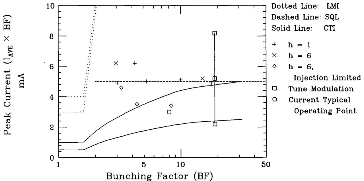
**Figure 1.** Threshold currents for various instabilities for electron cooled beams in the IUCF Cooler. These curves are based upon measurements and extrapolated according to theory.
