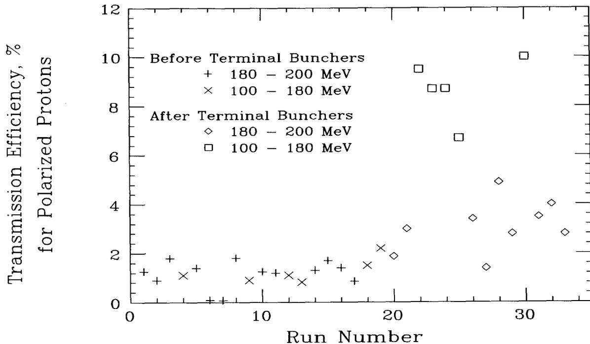
Figure 3. Effect of terminal bunchers. The numbers are from the operations logbook, not "typical" results obtained during beam studies.
