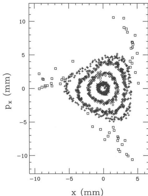
**Figure 2.** Poincaré map for motion near the 3<sup>rd</sup> integer resonance.
