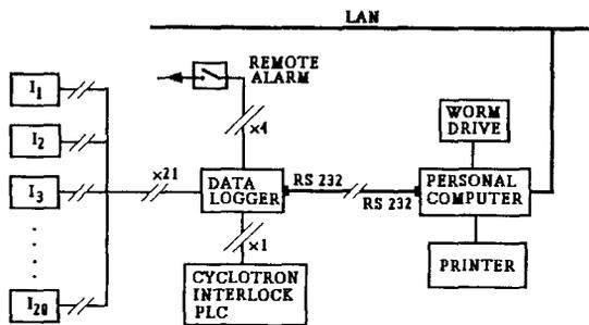
Fig. 5. Schematic Diagram of the Radiation Monitoring System showing the various Radiation monitors ( $I_1, I_2, \dots, I_{20}$ ), Datalogger, Remote alarms (x4), Cyclotron interlock PLC (x1) and the Computer system.
