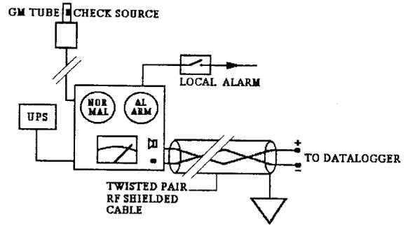
Fig. 4. Schematic Diagram of the basic Radiation Monitoring unit with its various components and Data and Alarm pathways.
