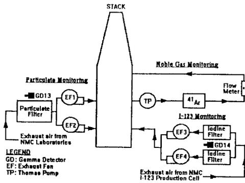
Fig. 2. Schematic Diagram of the Stack monitoring system showing the Filters, Radiation monitors and Pumps.
