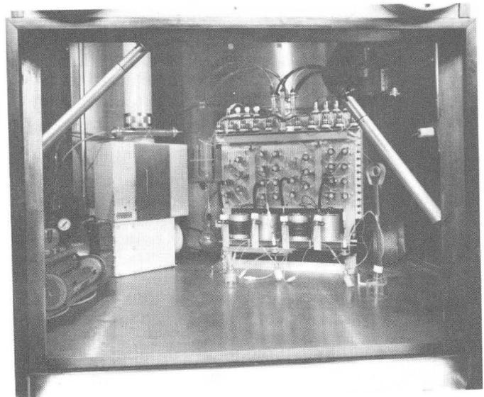
Fig. 4. A picture of the chemistry station mounted on a rack inside the hot cell. The two chemistry station are mounted side by side. The stations are cleaned and loaded with chemicals before the processing start each morning.
