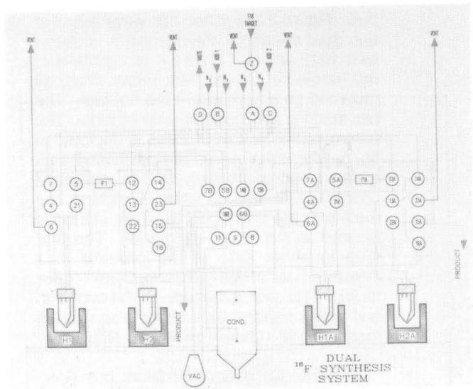
Fig. 3. A schematic drawing of the FDG dual processing chemistry station showing over forty Teflon valves. The first step in this process is to measure the radioactivity from the target.
