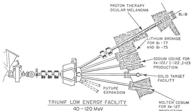
Fig.1. Beam line 2C (BL2C) and the four target stations used for radioisotope production.
