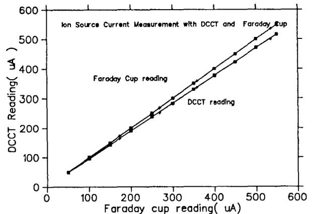
Fig.2. Ion current measured by Faraday Cup and DCCT
