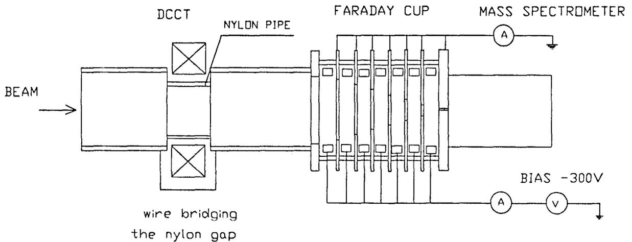
Fig. 1. IRM 2" cups ion source set up for DCCT test
