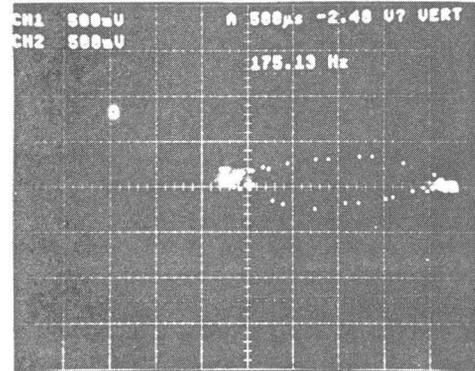
Figure 3. I-Q diagram showing the data clusters of demodulated beam phase signal. The distance between the two clusters is proportional to the magnitude of the beam current and the angle the beam phase.
