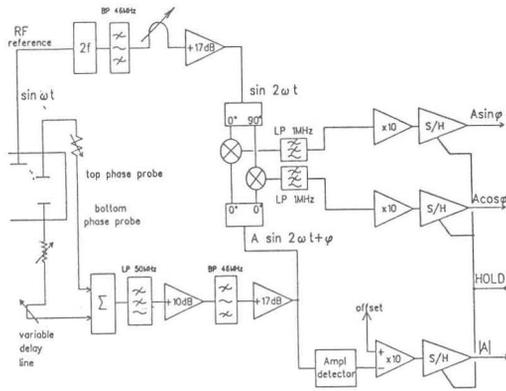
Figure 2. Block diagram of vector demodulator for the phase probe.
