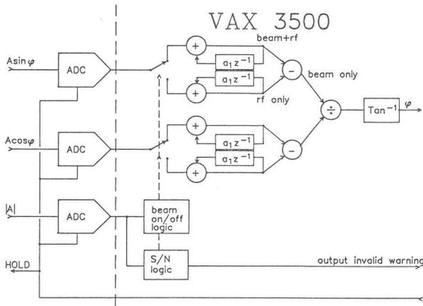
Figure 4. Software logic block diagram for the beam phase angle calculation.
