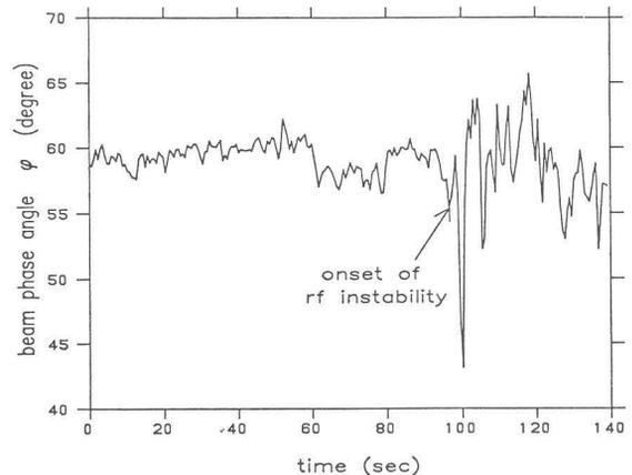
Figure 5. Beam phase angle before and after unstable rf operation.
