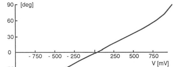
Fig. 9. Phase detection system output. This graph is obtained after phase detector output signal processing.
