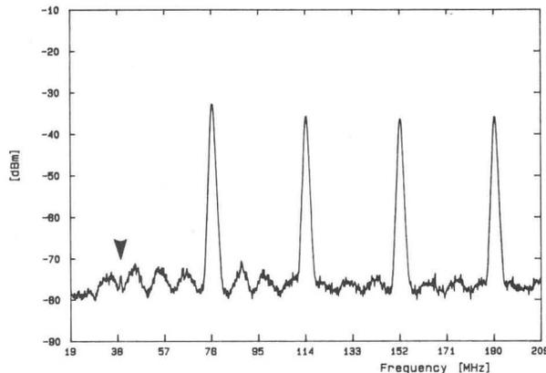
Fig. 8. Signal after interference filter. The arrow shows 1<sup>st</sup> harmonic power level.
