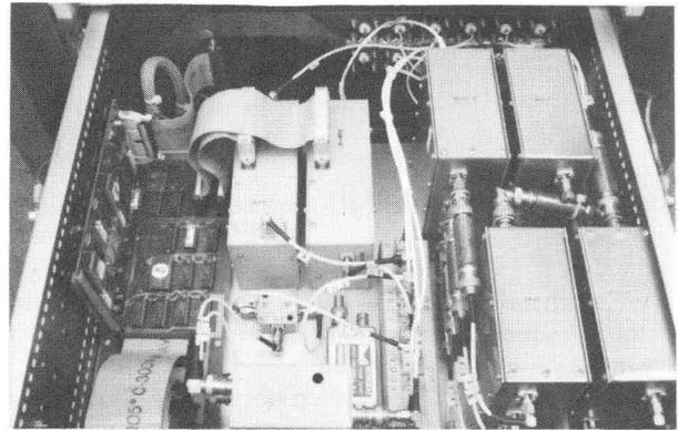
Fig.10. Internal layout of the phase detection section. Assembling techniques to reduce electromagnetic interference are shown.
