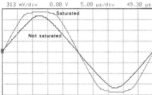
Fig. 6. Phase detector output characteristics, taken from a HP 54201A/D digitizing oscilloscope.
