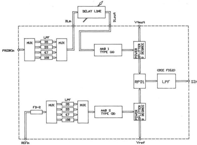
Fig. 5. Phase detection system. The frequency doubling system is also shown.
