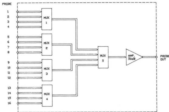
Fig. 3. Probe selection system. The 50 dB RF amplifier is also shown.
