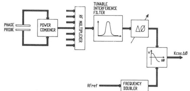
Fig. 2. Control Electronics block diagram.
