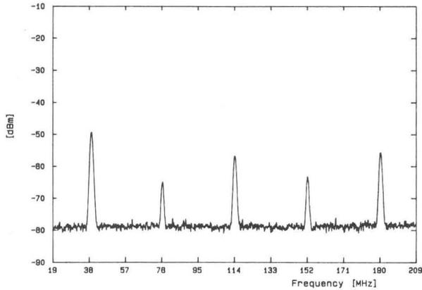
Fig. 7. Filter input signal spectrum. This signal is a simulation of a probe detected voltage when accelerating copper ions.
