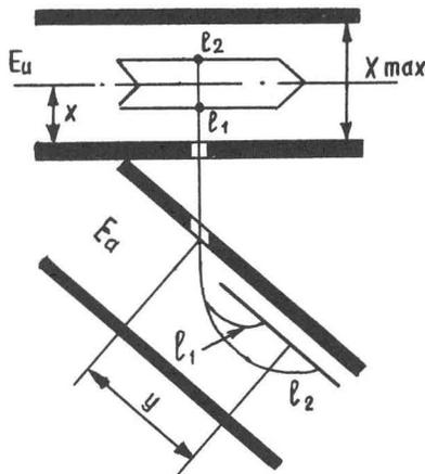
Fig.4. The transverse beam cross-section sensor diagram.
