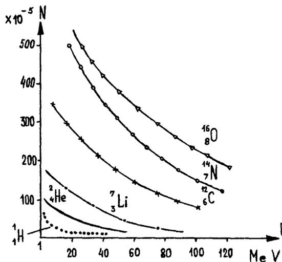
Fig.1. The calculated dependence of ionization power on a beam energy for various particles.
