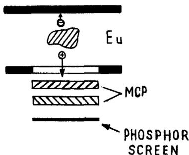
Fig.3. The cyclotron extracted beam profilometer.
