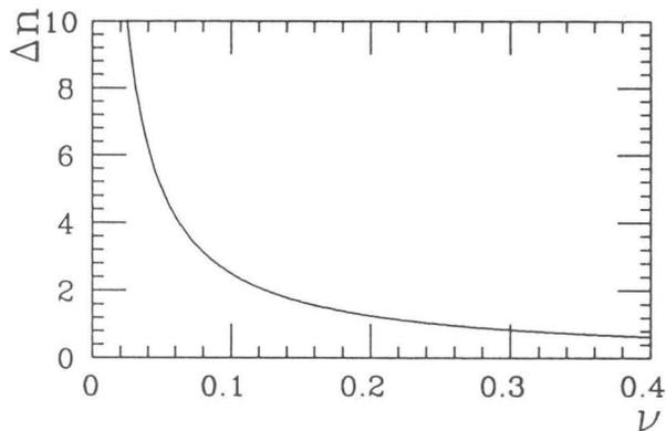
Fig. 2. The relative turns between two electric deflectors vs. the vertical tune with relatively well optimized conditions in eq. 21.
