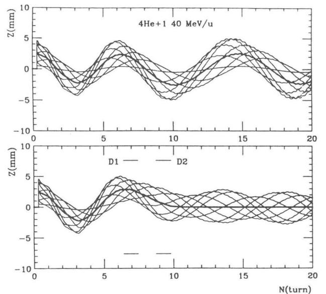
Fig. 5. Individual particle trajectories with different initial conditions as a function of turn number. A coherent vertical motion is simulated in the upper part. The lower part illustrates the calculated effect of the two vertical deflection plates. Also note that the central ray(the thick solid line) is on the median plane after passing the 2nd plate.
