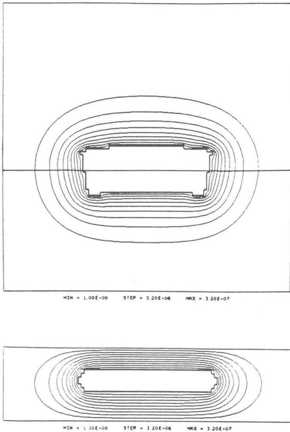
Fig. 3. A RELAX3D field calculation of a deflector plate showing equipotential lines both for top view(upper) and for cross sectional view(lower). The top solid line in the sectional view(lower) is the copper hill cover and the bottom solid line is the magnetic median plane.
