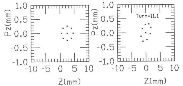
Fig. 4. Phase space coordinates of 9 rays at the beginning (left) and at turn=11.1 after passing the 2nd electric deflector(D2). The central ray has moved to the origin.
