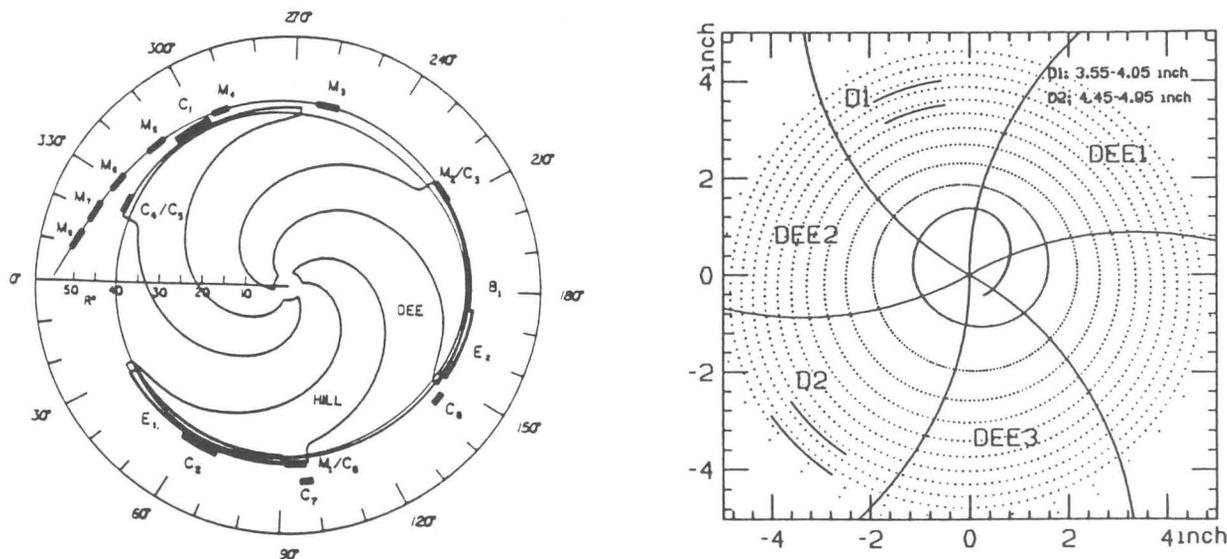
Fig. 1. Section view of the median plane of the K1200 cyclotron(left) and the enlarged top view of central region(right). The spiral dotted line shows a particle trajectory and D1, D2 are the electric deflectors locations.
