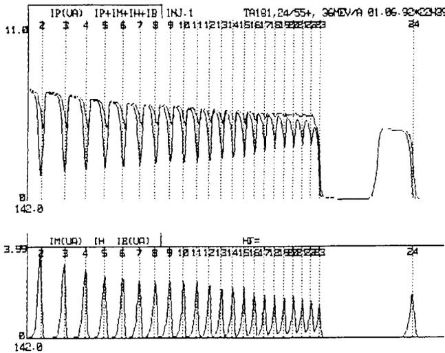
Figure 5 : Turn pattern of Ta in the cyclotron
