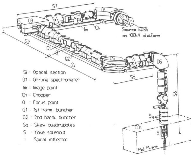
Figure 2 : General layout of the beam line
