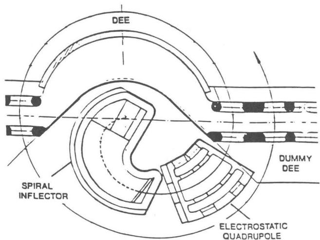
Figure 3 : Central region for the 100 kV injection
