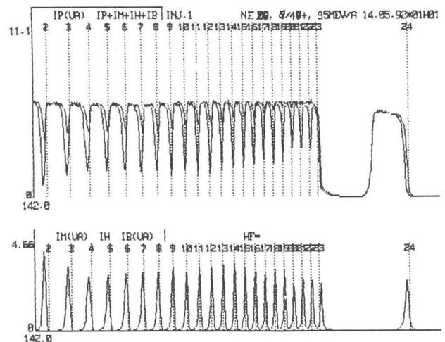
Figure 4 : Turn pattern of Ne in the cyclotron
