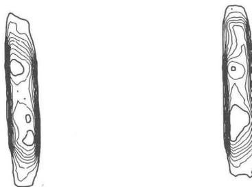
Figure 3. These two beam snapshots were taken at a radius of 0.51 m (left) and 0.52 m. The total vertical height as determined by the lowest contour line is 8.5 mm. It clearly shows the vertical oscillation of the beam and the radius gain of the beam between turns, for example on the left contour plot. The left edge of each contour plot corresponds to the edge of the scintillating plate, while the right edge is determined by the radius gain per turn and centering error.
