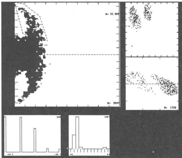
Figure 6. Snapshots of the computer screen showing a fenced area (dashed polygon) and the initial conditions and turn distribution of the selected particles.
