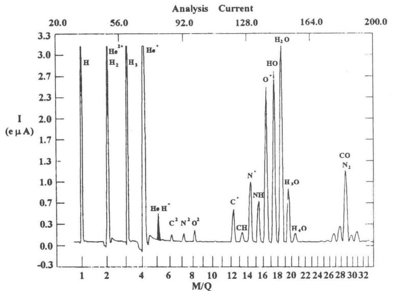
Figure 3. The He+H charge state distribution of the CPECR, showing the presence of the HeH<sup>+</sup> molecule, used to produce low energy H beams in the K1200 cyclotron.
