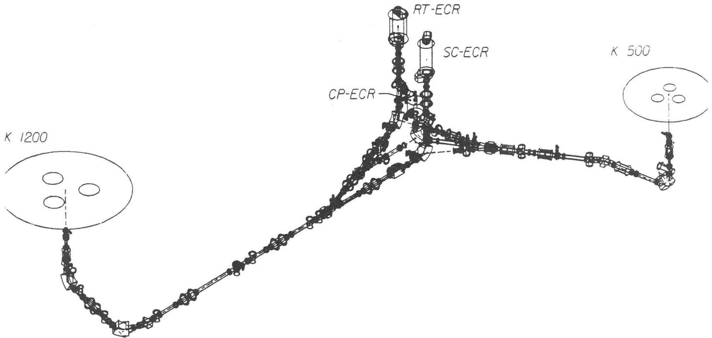
Figure 1. The beam development system at NSCL consists of ECR sources, injections and the superconducting cyclotrons.
