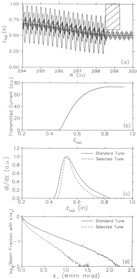
Figure 5: A schematic summarizing the foil dip method for determining vertical beam width and emittance. The beam transmitted (a) past the foil of height  $z$  is measured (b) and the result can be differentiated to produce the vertical half width (c) or plotted on a log scale to show the fraction of the beam lying outside a given emittance (d).
