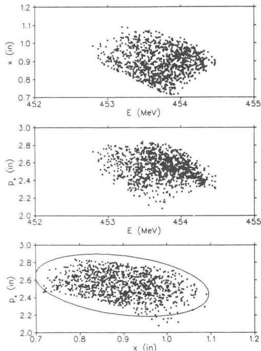
Figure 1: COMA simulation result showing the final position of particles in  $E - x$ ,  $E - p_x$  and  $x - p_x$  phase spaces for a beam with circulating radial emittance of  $1\pi\mu\text{m}$ , phase band of  $40^\circ$ , and RFD voltage of  $110\text{ V/mm-m}$ . An ellipse of  $4\pi\mu\text{m}$  encloses 99% of the extracted particles.
