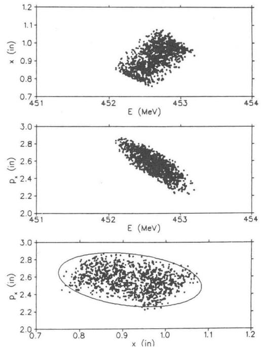
Figure 2: COMA simulation same as for study summarized in Fig. 1 only with flattopping cavity powered (18 kV) to reduce phase dependent effects. An ellipse of  $3\pi\mu\text{m}$  encloses 99% of the extracted particles.
