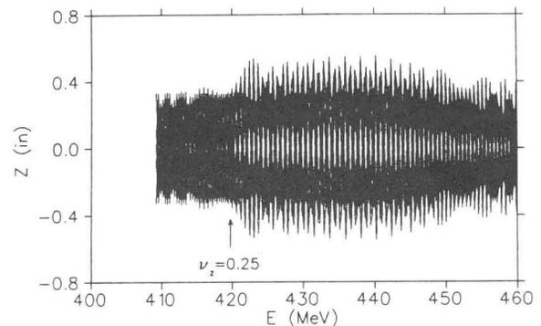
Figure 3: Result of GOBLIN simulation showing the vertical beam envelope at one azimuth while accelerating through the RFD. A growth of 50% occurs as the RFD is entered for an RFD strength of  $110\text{ V/mm-m}$ .
