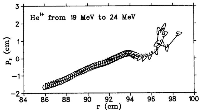
Fig. 5. Radial phase space of a  $\text{He}^{1+}$  beam prior to extraction at  $\theta = 280$  deg. The tracked particles started at an energy of 10 MeV and at the same RF phase (0 deg) on an eigen ellipse.
