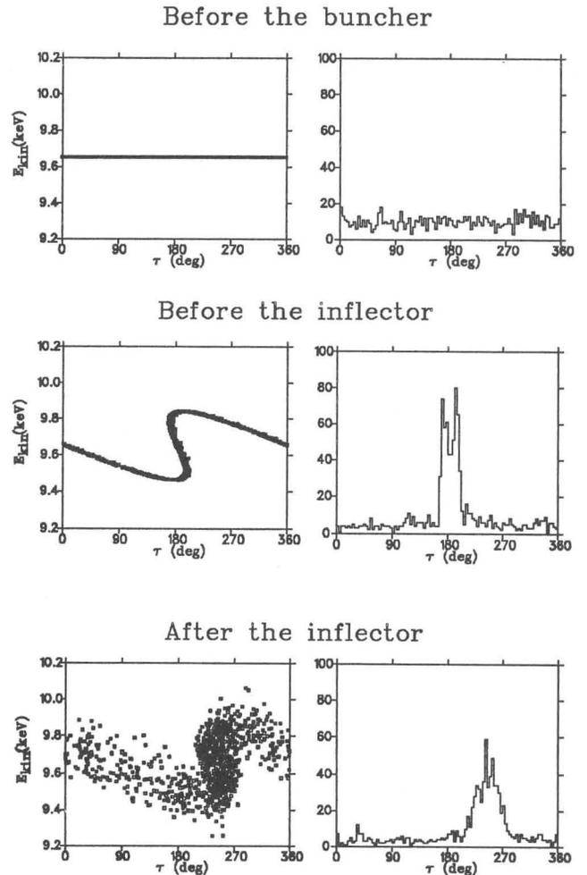
Fig. 3. Beam simulation with the buncher, before the buncher (above), before the inflector (middle) and after the inflector (below).
