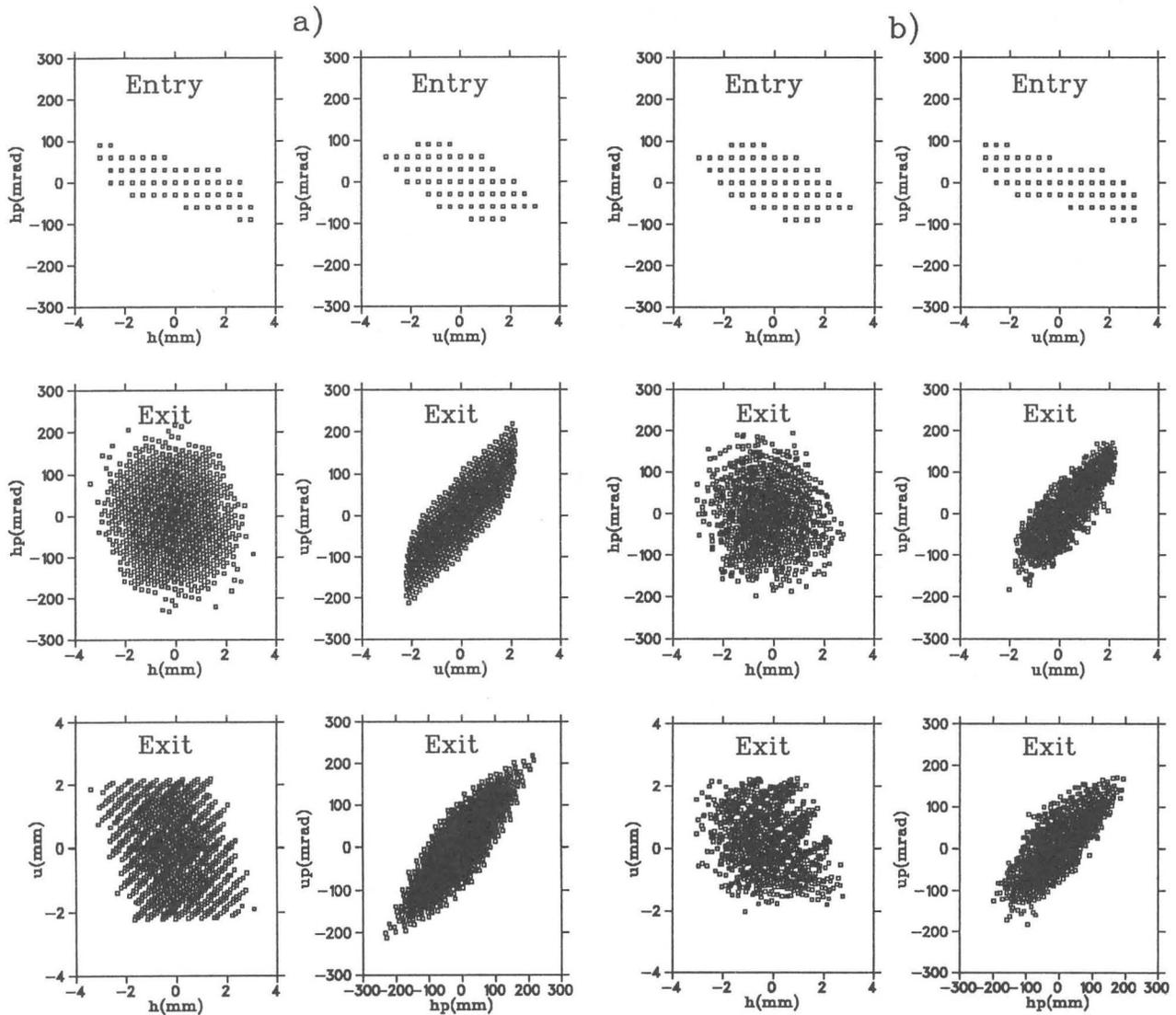
Fig. 4. The transverse acceptances (entry) of the second harmonic inflector using a) transfer matrices, and b) tracking particles with ION\_TRACKER. Each point in the entry sub phase space contains several particles: same  $(h, hp)$  but different  $(u, up)$  and vice-versa.
