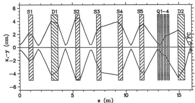
Fig. 1. The injection line elements and beam envelopes.
