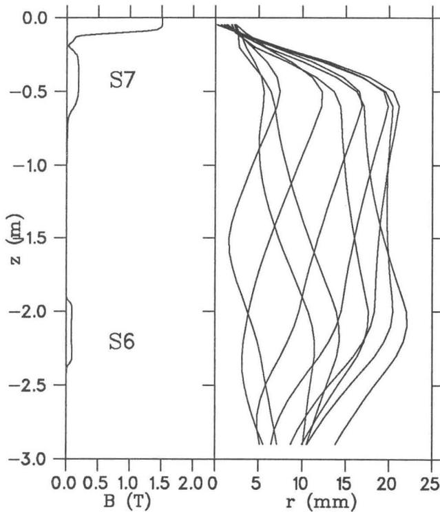
Fig. 2. Tracked beam in the axial hole of the K130 cyclotron and the corresponding axial magnetic field with solenoids S6 and S7.
