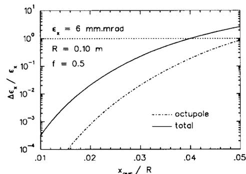
Figure 3. Relative change of emittance in the  $x$ -direction as a function of scaled rms beam radius for a smooth hill or valley field profile.
