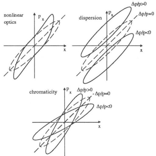
Figure 1. A graphical illustration of three causes for emittance growth
