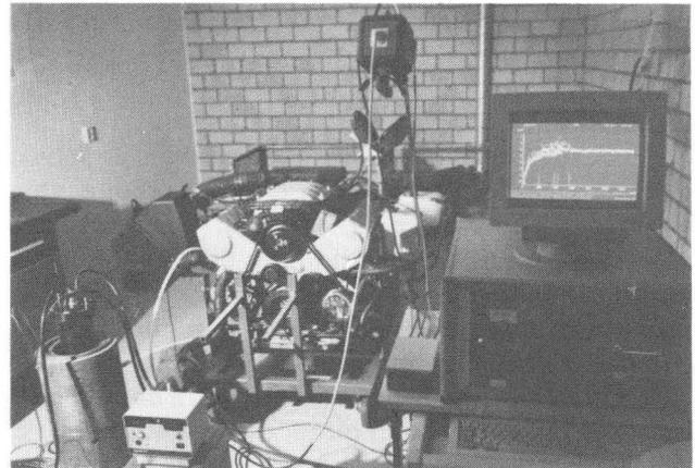
Fig. 3: The wear behavior of Be-7 labelled parts, a gear of Polyamid and a crankshaft seal of Viton (Elastomer), have been measured under real operation conditions in a high-powered engine of Audi on a test bench at the Fa. Heß, as illustrated by the picture. Demonstration measurements and material testing have been performed in cooperation with the Company Audi and Fa. Heß, Ingolstadt.
