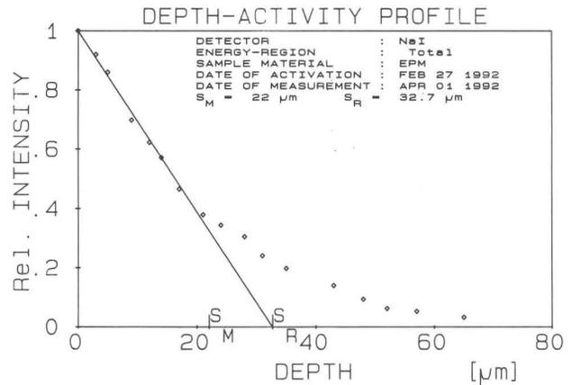
Fig. 2: The activity over depth distribution of implanted Be-7 in EPM-Polyamid is demonstrating the quality of the radioactive labelling by the linear region of 20  $\mu\text{m}$  near the surface suitable for wear measurements.
