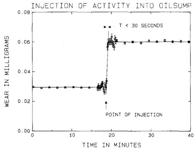
Fig. 6 : For the demonstration of the sensitivity and reactivity of RTM wear diagnosis a definite activity - representing 30 µg wear mass - was injected in the oil sump of the operated engine on the KfK test bench. The applied concentration measurement device registered the full wear mass 30 sec after the injection. A wear mass down to 10 µg - corresponding to a linear wear of several nanometers - can distinctly be resolved.
