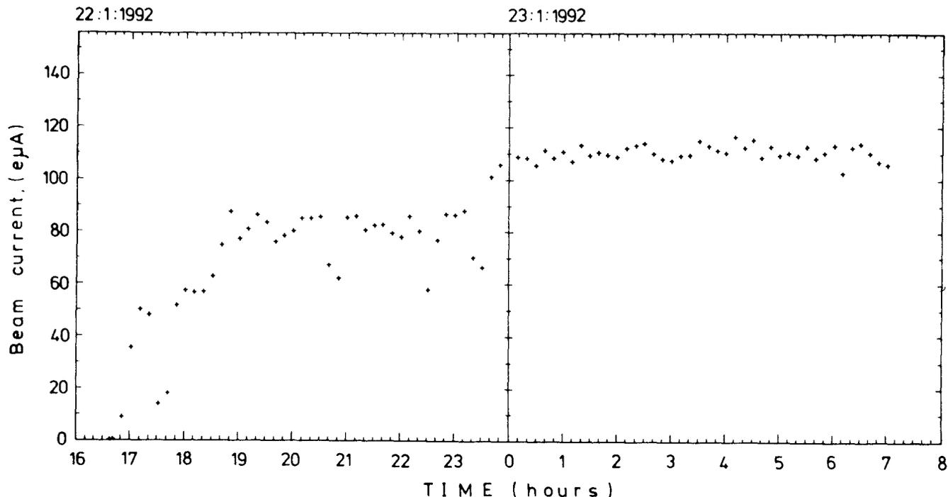
Fig. 3 The record of a target current during irradiation.
