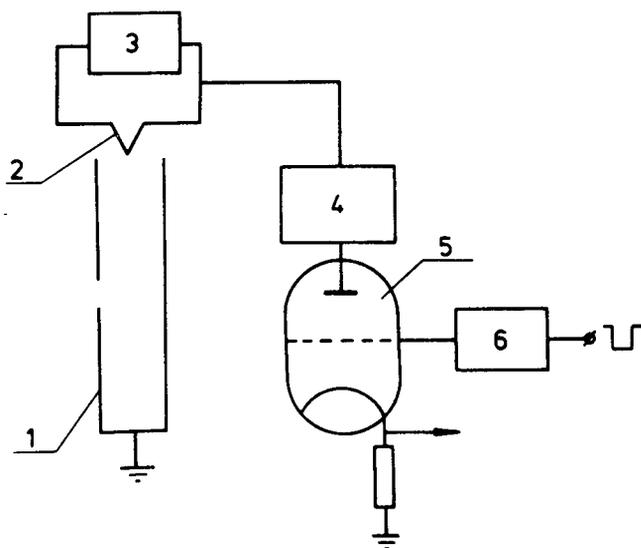
Fig. 2. The power supply circuit of the ion source: 1-discharge chamber (anode), 2-cathode, 3-cathode power supply, 4-discharge power supply, 5-modulating valve, 6-amplifier.
