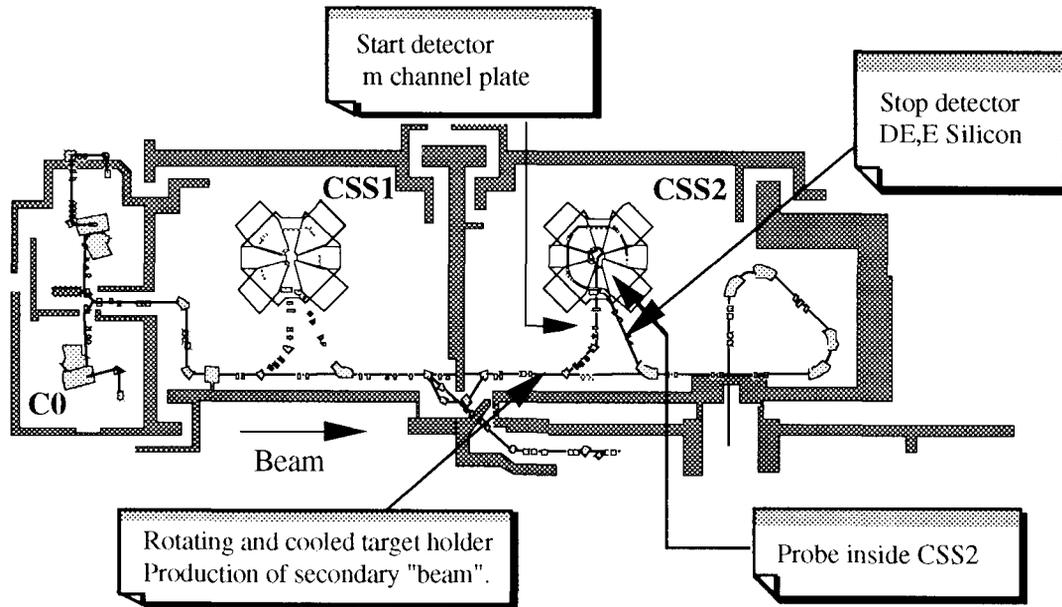
Fig. 1 Schematic view of the GANIL cyclotron facility. The principal component locations used for the mass measurements are indicated.
