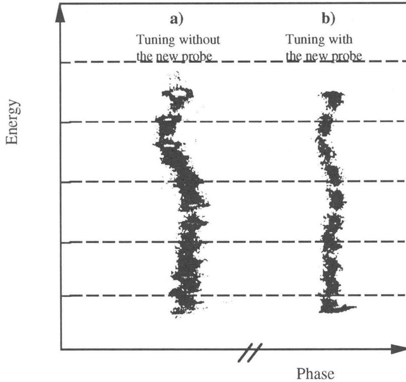
Fig. 3 Phase space diagram of the particles in the cyclotron. Fig. 3a shows the phase space obtained just after the prior tuning using a particle having the same  $A/q$  ratio as the nuclei of interest. Fig. 3b shows the final phase space using this detector for the fine tuning of the magnetic field.
