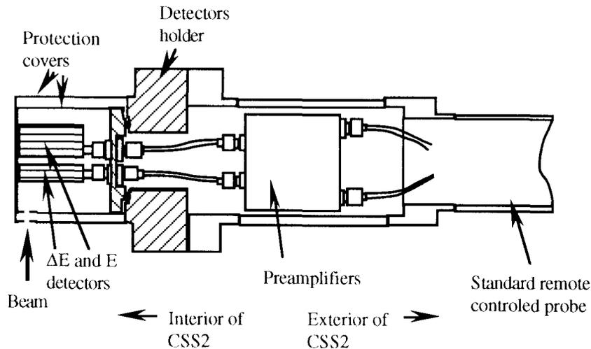
Fig. 2 Schematic of the probe installed in one sector of the CSS2.
