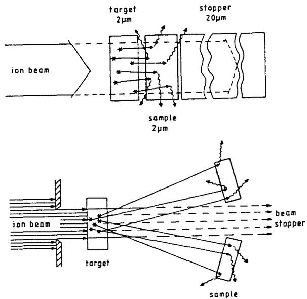
Figure 4 Experimental arrangements for recoil implantation.
