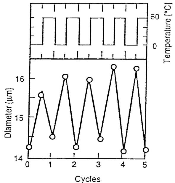
Figure 6 Change in size of pores formed in a thermally responsive film when cycled between  $0^\circ\text{C}$  and  $60^\circ\text{C}$ .
