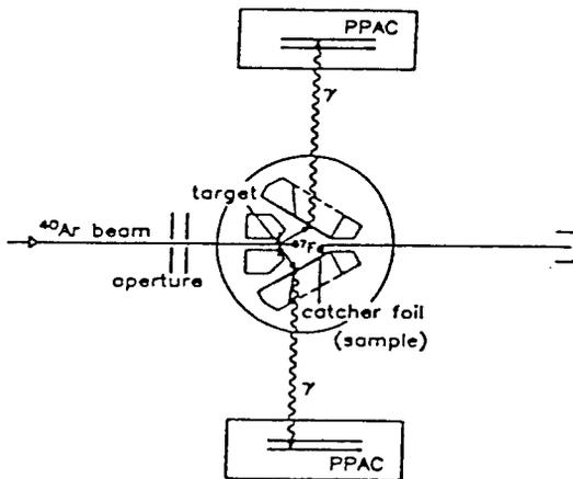
Figure 5 Sketch of the experimental setup for "in beam Mössbauer spectroscopy". PPAC stands for parallel plate avalanche counter.
