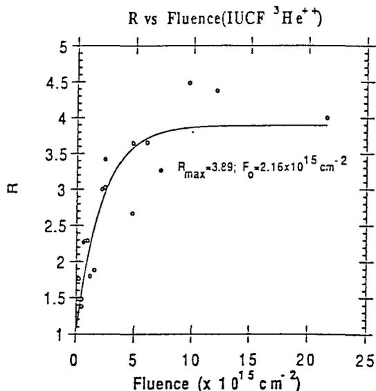
Figure 7 Ratio R of trapped field after to trapped field before irradiation versus particle fluence.
