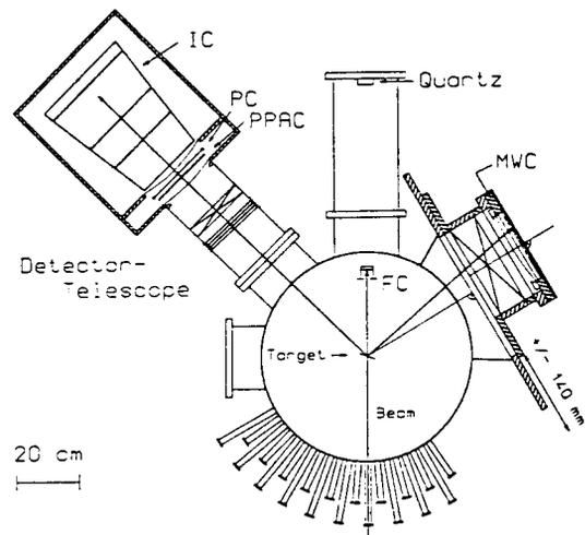
Figure 1 Sketch of the experimental ERDA setup. The scattering chamber is mounted on a rotatable support, with two large-area detectors attached.
