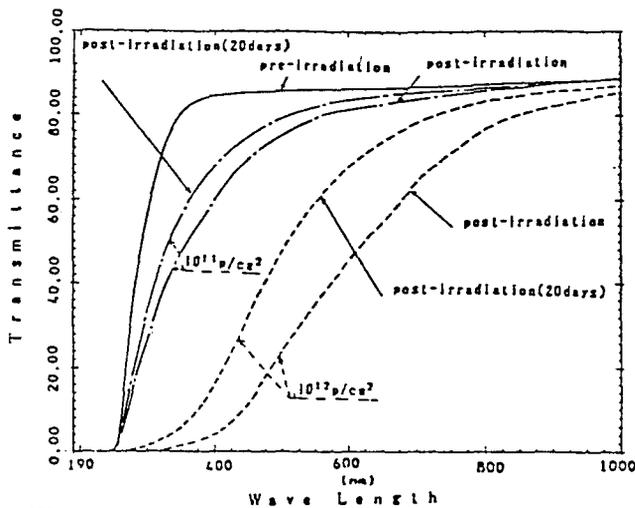
Figure 3 Transmission curves of optical glass before and after 40 MeV proton irradiation.
