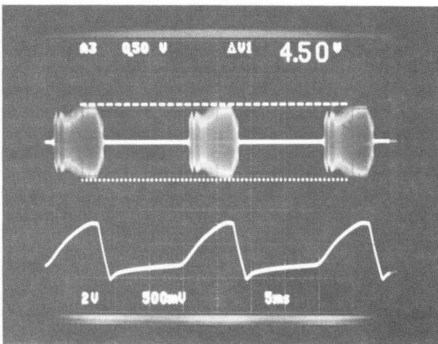
Fig. 5. High power operation of rf cavity using perpendicularly biased ferrite. The top trace shows voltage at the accelerating gap (dashed lines indicate 65 kV), the lower trace the bias power supply current.
