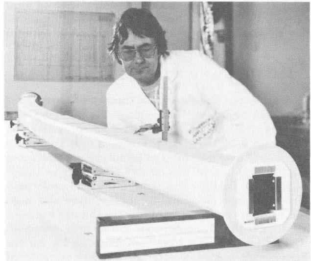
Fig. 6. Ceramic pipe and wire shield (RAL design).
