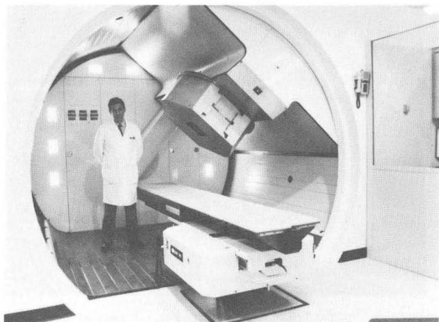
Figure 4. The Harper Cyclotron as it appears to a patient arriving for therapy. The large object above the patient table is the neutron collimator consisting of 12,000 adjustable 3 mm dia. Tungsten rods.
