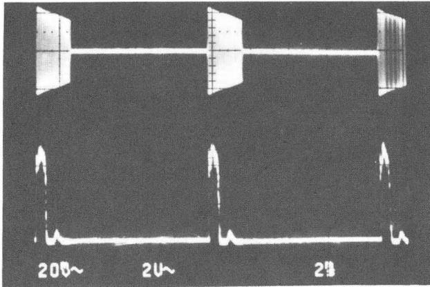
Figure 6. Dual beam scope trace from an rf pickup loop (top) and from the full energy target (bottom) showing three 2 millisecond 100 Herz pulses on a 2 ms/cm time scale. Time average beam  $12\mu\text{a}$ .
