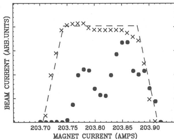
Figure 5. Plot of target current vs. magnet current with target at 286 millimeter for the x data and 298 millimeters for the circle data. The dashed line is the expected 286 millimeter curve.
