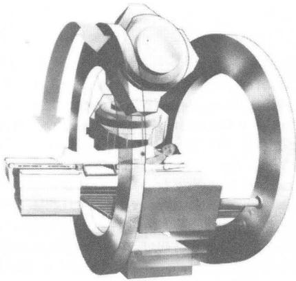
Figure 1. Schematic view of the Harper Hospital neutron therapy system showing the cyclotron mounted between two large rings which move it on a vertical arc about the patient.
