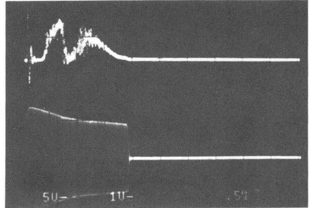
Figure 8. Scope trace similar to Fig. 7 except a further adjustment of the dee fine tuner has moved the first target current peak away from the origin and changed the time average beam current to  $8.4\mu\text{a}$ .
