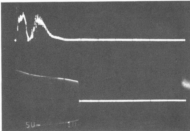
Figure 7. Target current and dee volts on an expanded time scale (0.5 ms/cm) with the dee fine tuner shifted slightly relative to Fig. 6 and with the target trace on the upper scale. This setting reduced the beam current to  $9.2\mu\text{a}$  and changed the two target current peaks to approximately equal magnitude.
