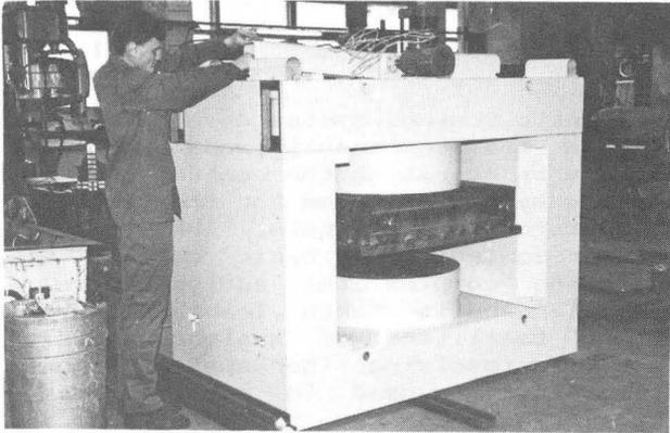
Fig. 2. Yoke and poles of MPC-10 magnetic system.
