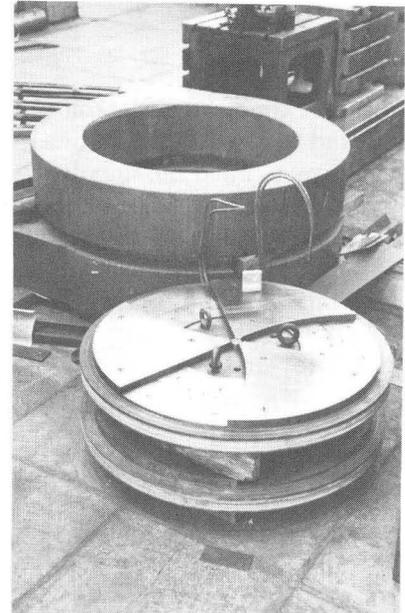
Fig. 1. Magnet structure and main coils.
