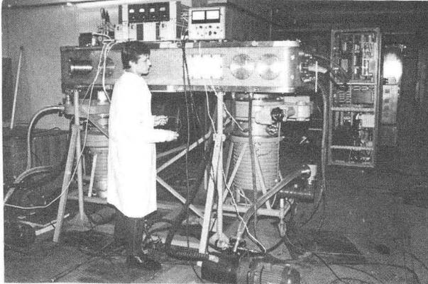
Fig. 4. Vacuum tests of the cyclotron chamber.
