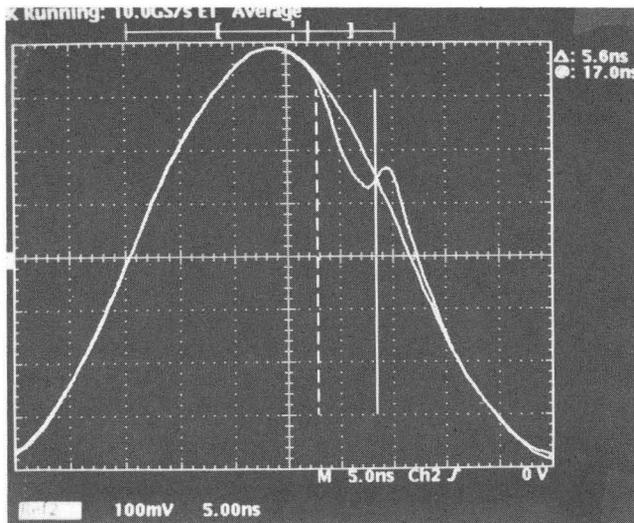
Fig. 4. Typical beam signals measured by the phase probe(CH10) in case of 70 MeV protons.
