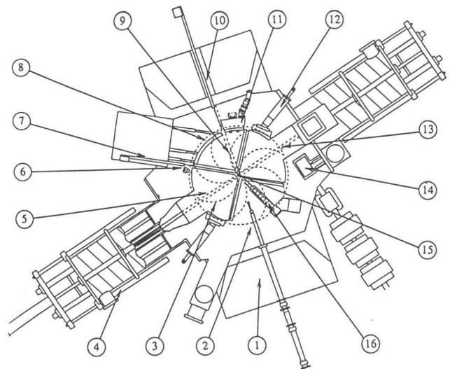
(1) Yoke, (2) Main probe, (3) Dee, (4) Resonator, (5) Puller, (6) Dee voltage pickup, (7) Deflector probe, (8) Deflector, (9) Phase slit(II), (10) Magnetic channel probe, (11) Magnetic channel, (12) Capacitive frequency tuner, (13) Phase slit(I), (14) Gradient corrector, (15) Inflector, (16) Phase probe
