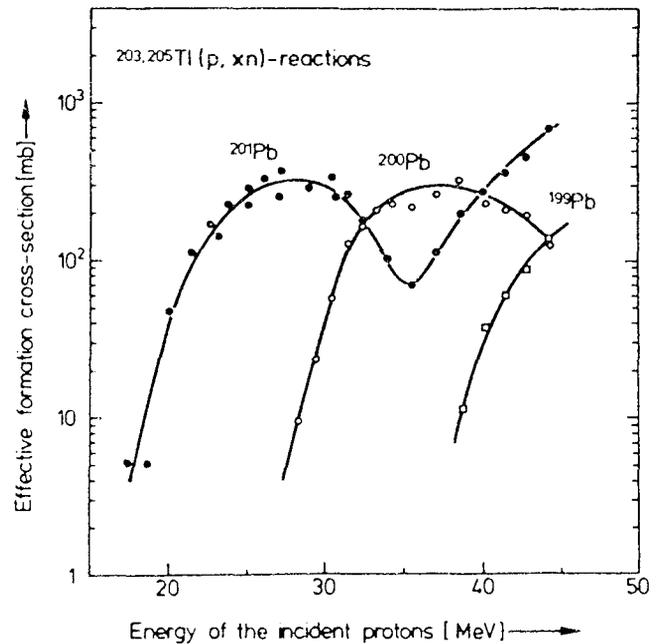
Fig. 3: Cross section for the nuclear reaction Tl-203(p,3n) taken from ref. 2
