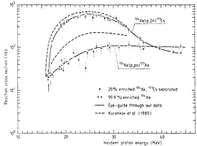
Fig. 2: Cross section for I-123 via Xe-124(p,2n) taken from ref. 1
