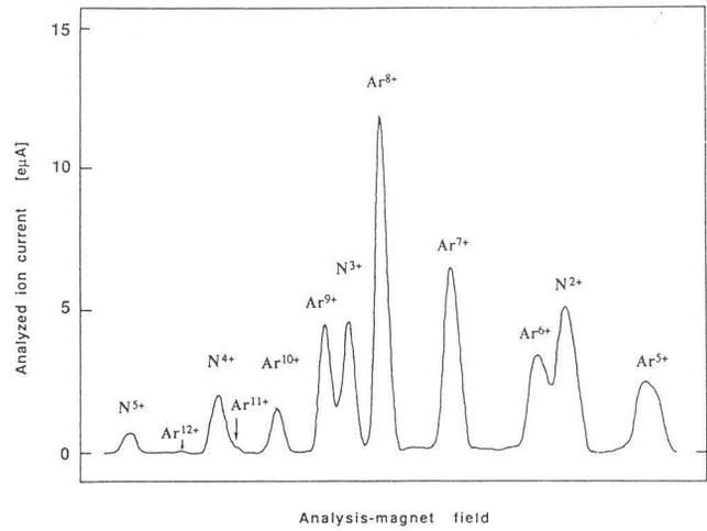
Fig. 2. Charge state distribution of argon ions analyzed with a 90-degree magnet.
