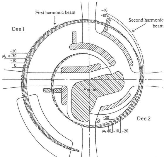
Fig. 1. Central region in the CW case with internal ion source. Double arc anode permits operation both with first and second harmonic.
