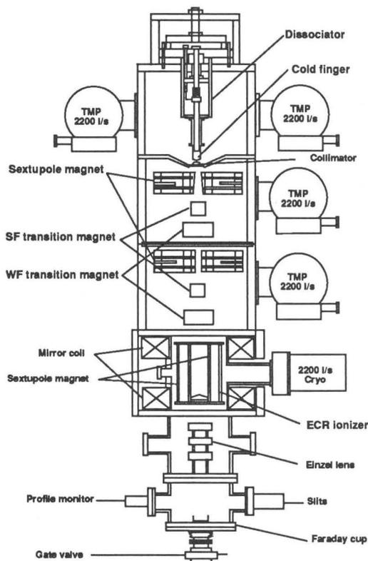
Fig.4. Schematic side view of the polarized ion source.
