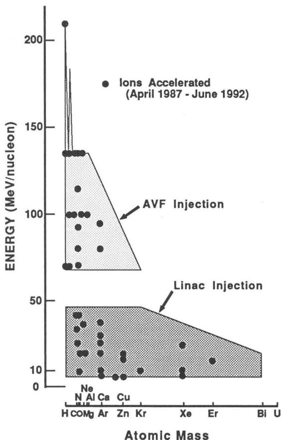
Fig. 3. Energy-Mass curve for the RRC; beams delivered for users are plotted.
