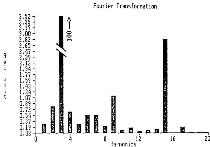
Fig.3. The Fourier-spectra of the radial field component at a given axial position inside a NdFeB hexapole magnet (region: 0-360°, R=33 mm).
