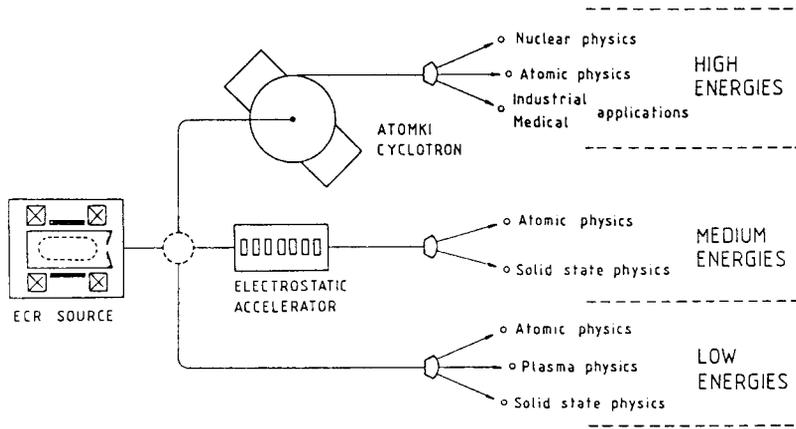
Fig.1. The scheme of the proposed heavy ion facility.
