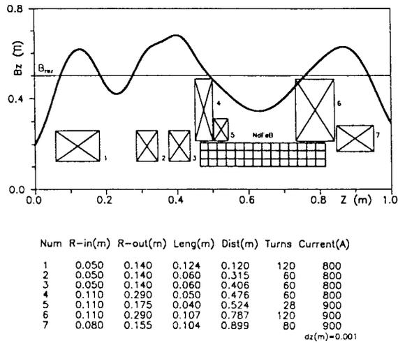
Fig.2. Axial magnetic field on the axis of the ECR ion source and coil parameters.
