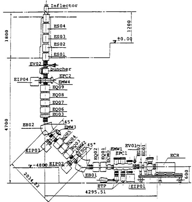
Fig.4 Beam line from ECR ion source to the inflector.
