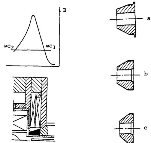
Fig.2. Conical iron ring and the axial field distribution.
