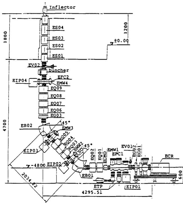
Fig.2. The beam transfer line from ECR ion source to the center of SFC
