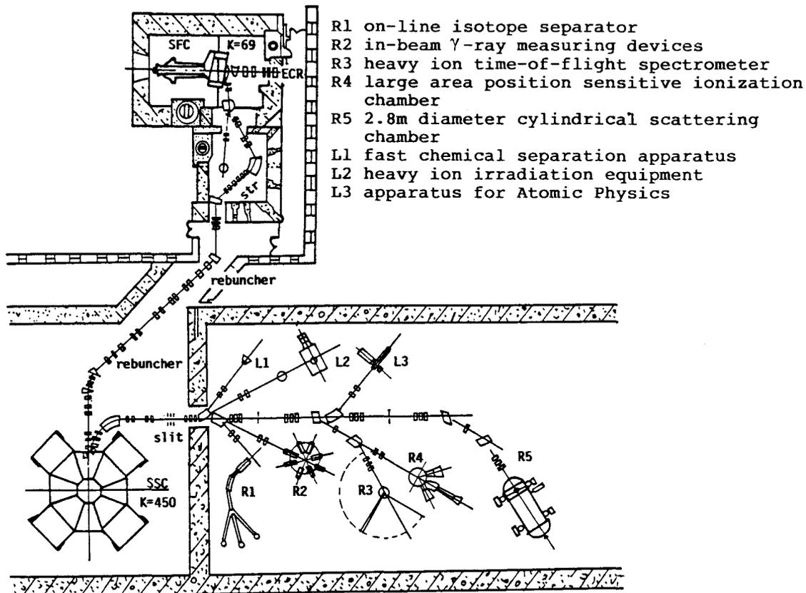
Fig.1. The general layout of HIRFL. R1- Isotope Separator, R2- In Beam Gamma-ray Measuring Device, R3- Heavy Ion Telescope, R4- Large Area Position Sensitive Ionization Chamber, R5- Heavy Ion Scattering Chamber, L1- Fast Chemical Separation Apparatus, L2- Irradiation Terminal, L3- Atomic Physics Terminal.
