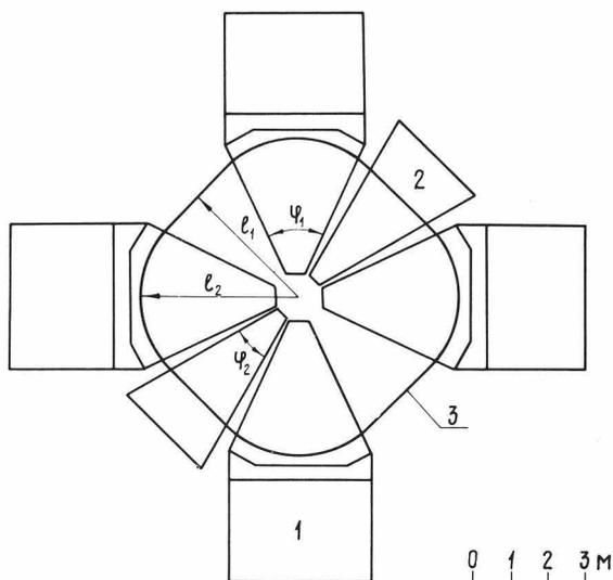
Fig. 5. Simplified scheme of separated sector cyclotron: 1-sector,  $\varphi_1=50^\circ$ , 2-dee,  $\varphi_2=30^\circ$ , 3-equilibrium orbit.
