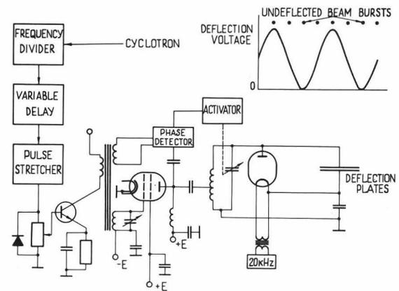
Fig. 4. Simplified scheme of particles bursts selection system.
