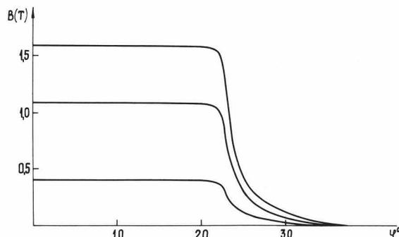
Fig. 7. Azimuthal distribution of magnetic field in the median plane.
