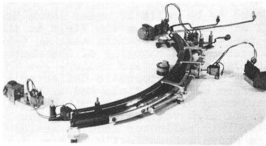
Fig. 2. General view of the adjustable deflector.
