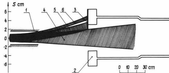
Fig. 3. Particles bursts sweeping off system and beam envelopes: 1-RF selector, 2-beamline, 3-collimator, 4,5,6-beams at potential difference of 0, 15 kV and 30 kV.
