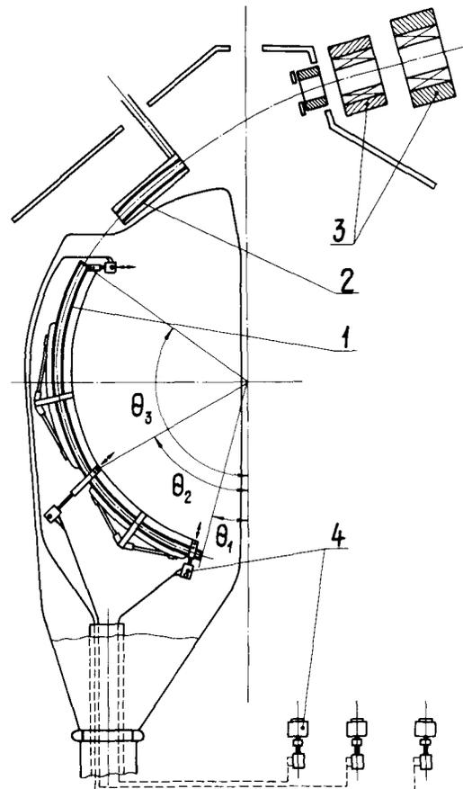
Fig. 1. The beam extraction system: 1-adjustable deflector, 2-additional deflector, 3-steering magnets, 4-hydraulic cylinders.
