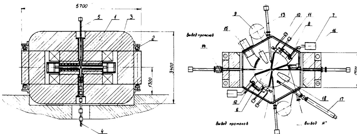
Fig. 1. General view of cyclotron. 1 - Electromagnet, 2 - Hydraulic jack, 3 - Vacuum chamber, 4 - External injection system, 5 - Axial injection deflector, 6 - Resonance system (dee), 7 - Final cascade of RF generator, 8 - RF power input, 9 - Vacuum pump, 10 - Tuning condenser, 11 - Trimmer of automatic frequency tuning, 12 - RF probe, 13 - Diagnostics probe, 14 - Septum protection foil, 15 - Extraction system deflector, 16 - Magnetic channel, 17 - Stripping device, 18 - Cryopanel.
