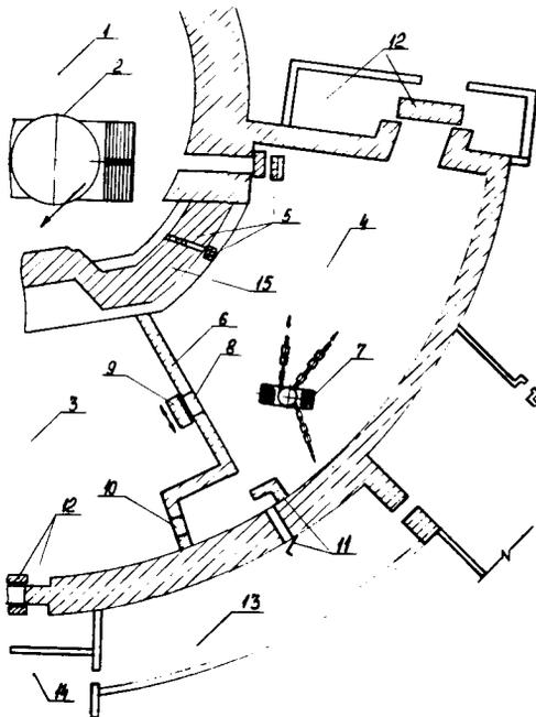
Fig. 2. Scheme of cyclotron arrangement. 1 - Hall of synchrocyclotron, 2 - Synchrocyclotron, 3 - Experimental hall, 4 - Cyclotron hall, 5 - Additional shielding, 6 - Wall separating the cyclotron hall, 7 - Cyclotron, 8 - Opening for crane passage closed by a wheeled block, 9 - Crane cargo opening, 10 - Cyclotron hall entrance, 12 - Shielding doors, 13 - Control hall, 14 - Laboratories, 15 - Shielding wall from iron block.
