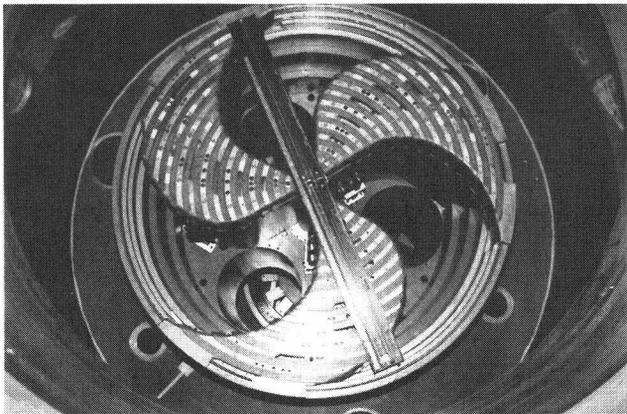
Figure 2. The lower pole with correction coils and field mapper.
