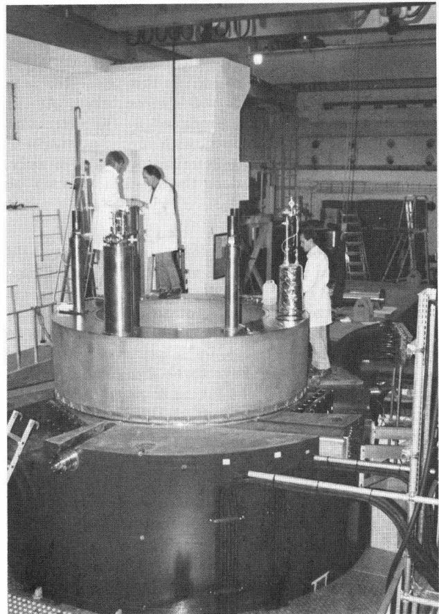
Figure 3. The cryostat, placed in the lower half of the yoke.
