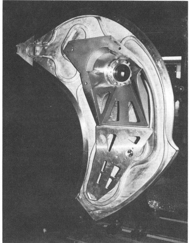
Fig.7. Interior view of acceleration electrode.
