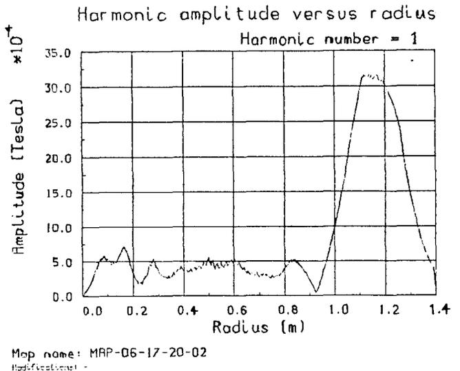
Fig.5. Measured field at  $B_0 = 2.2 T$ : first harmonic amplitude as a function of radius.
