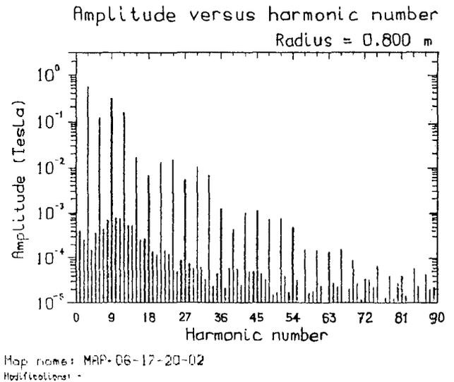
Fig.4. Measured field at  $B_0 = 2.2 T$ : spectral analysis at  $r=0.8 m$ .
