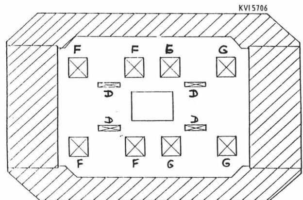
Fig.12. Cross-section of the focussing channel at the location of the first active element. F and G are gradient coils, D indicates dipole coils
