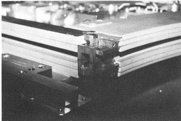
Fig.11. EMC-1: Detail of conductor lay-out at the channel exit.
