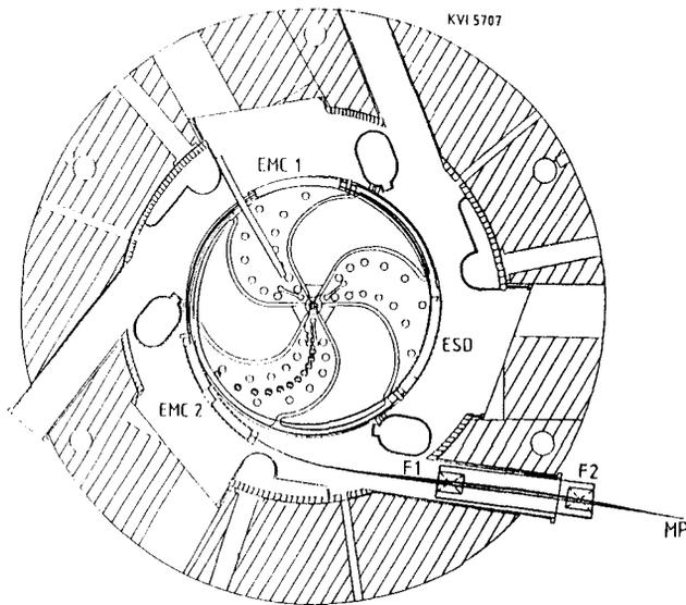
Fig.8. Midplane section of AGOR, showing location of the extraction channels.
