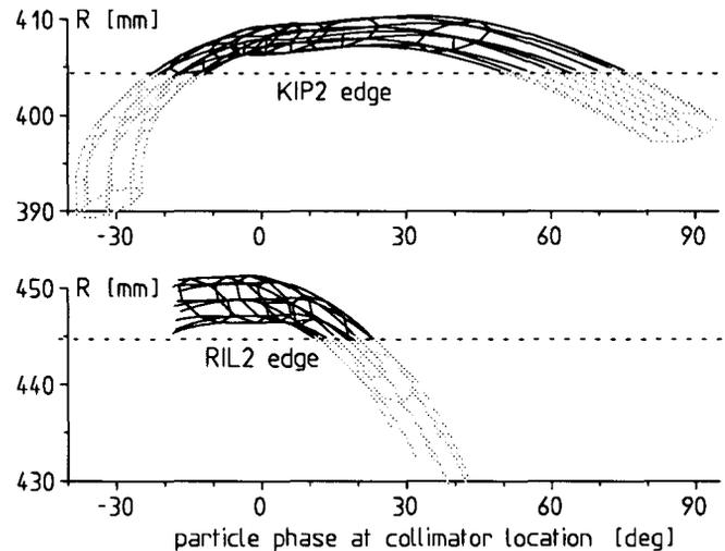
Fig. 4. Phasespace cutting by the radial collimators KIP2 and RIL2 for a SCL bunched beam. The radial and phase distribution of a simulated beam before (faint lines) and after (solid lines) being cut by KIP2 (135°) and by the new collimator RIL2 (235°).
