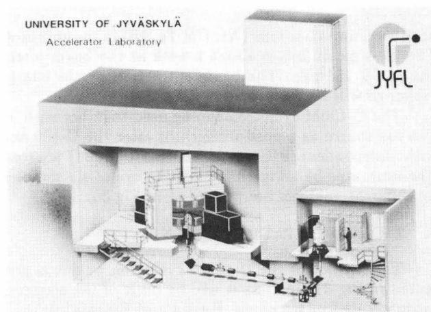
Fig. 1. Three-dimensional sketch of the K130 cyclotron with the ECR ion source and injection line.
