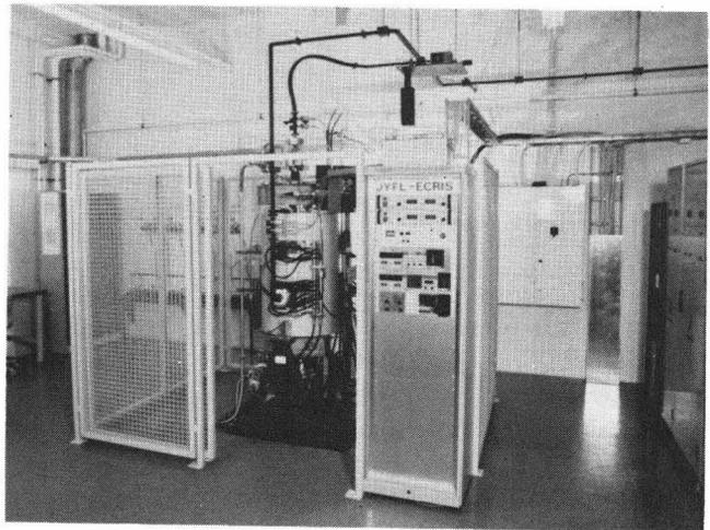
Fig. 3. Photo of the ECR ion source inside the HV protection fence.
