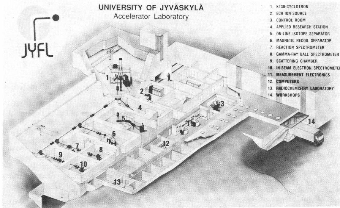
Fig. 6. Lay-out of the laboratory.
