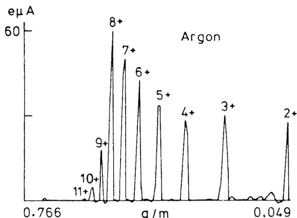
Fig. 4. Charge-state distribution of argon extracted at 10 kV. Microwave input power: 1st stage 16 W, 2nd stage 62 W.
