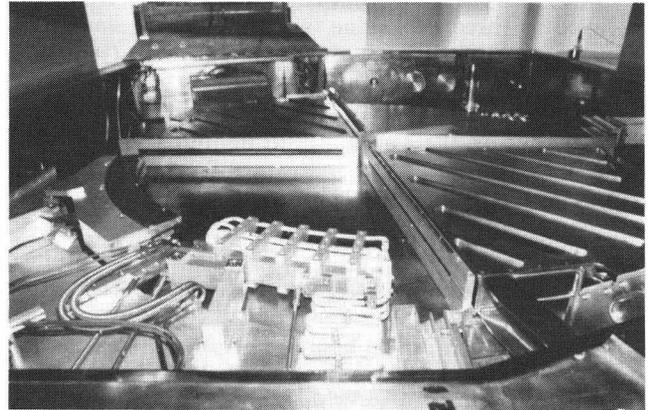
Fig. 2. Accelerator chamber of the K130 cyclotron. The extractor is in front. The phase probes and the central region were not installed in this photo.
