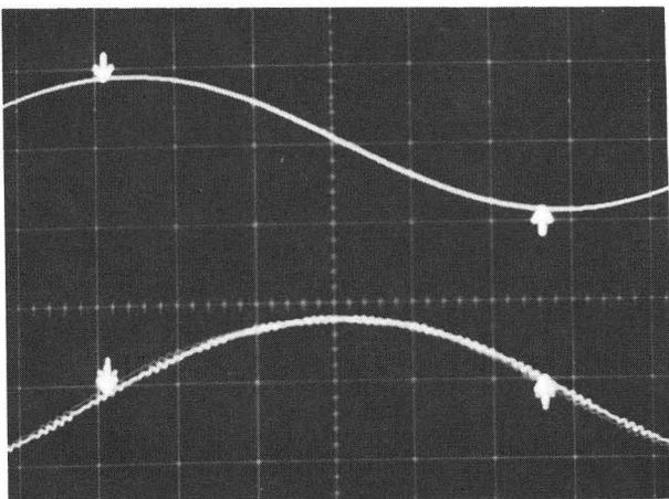
Fig. 9. Relative beam phase for few nA beams. Upper and lower correspond to pre-injection beam and pre-extraction beam, respectively. The IF phase signals are averaged by digital oscilloscope.  $20^\circ/\text{div}$ .
