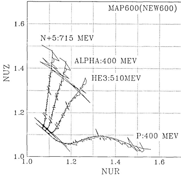
Fig. 5. Comparison between betatron frequencies calculated from the measured field and the designed one.
