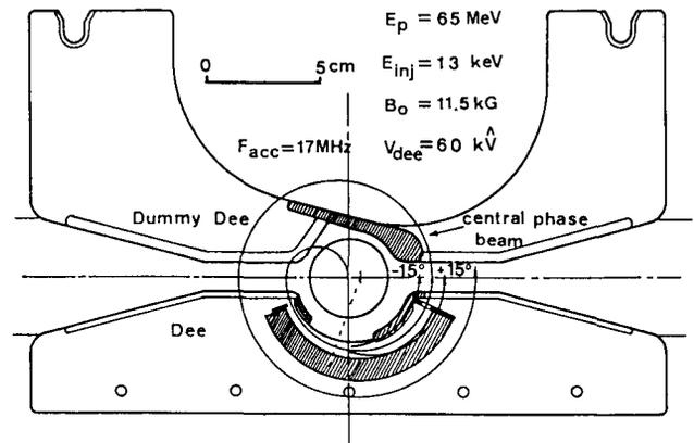
Fig. 7. Beam phase selector for axial injection mode of the AVF cyclotron.
