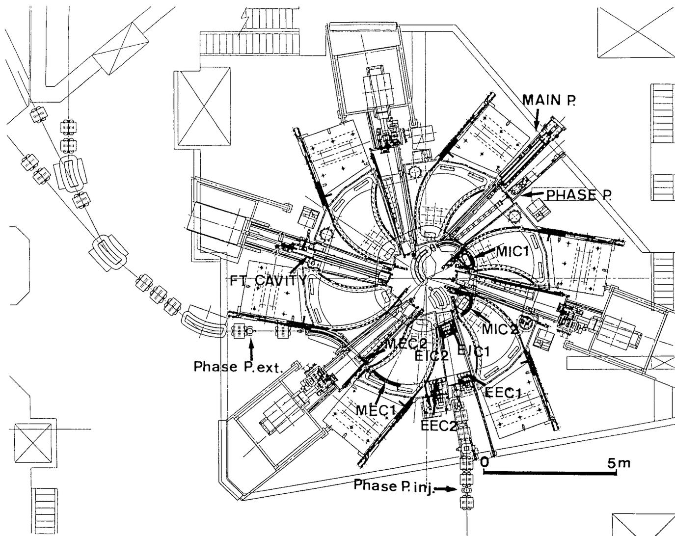
Fig. 2. Plan view of the ring cyclotron.
