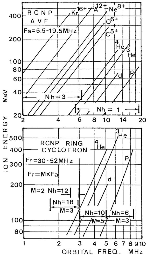
Fig. 3. Orbital frequencies, acceleration frequencies ( $F_a$  &  $F_r$ ) and harmonic numbers of acceleration ( $N_h$ ) in the RCNP AVF cyclotron and the RCNP ring cyclotron for various ions and energies.  $M$  is ratio of the acceleration frequency of the ring cyclotron to the AVF cyclotron.
