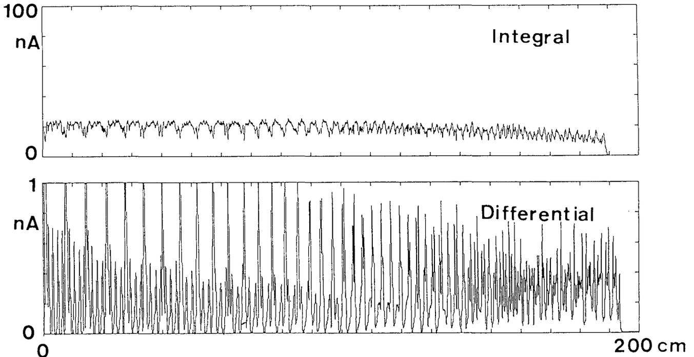
Fig. 8. Turn pattern measured by a main probe.
