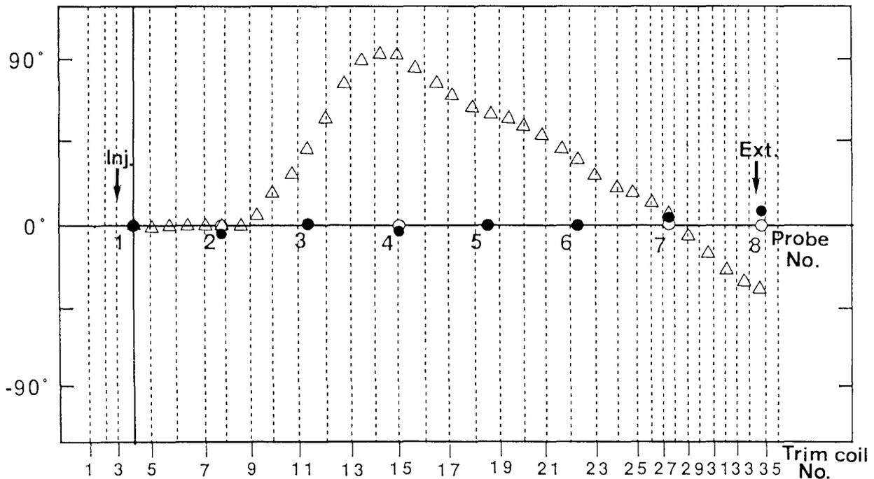
Fig. 6. Measured beam phase on predicted trim coil currents and optimized isochronous field, for 300 MeV proton acceleration.
