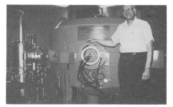
Fig.29 The MINI-Cyclotron (K20) at BNL, made by Japan Steel Works. They also made many BABY Cyclotrons (K14) in hospitals.
