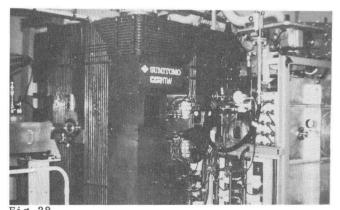
Fig.28 The CYRIC cyclotron (K50) at Tohoku Univ., completed in 1978, which was made by Sumitomo Heavy Industries with a technical cooperation with CGR MeV. They also made many other cyclotrons named CYPRIS (K70, K20, K16) for isotope production.
