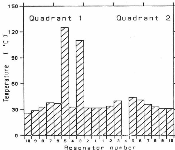
Fig. 6. Temperatures of strongbacks in normal operation. In quadrant 1 only segments 3 and 5 have leakage voltages suitable for multipactoring, in this case.
