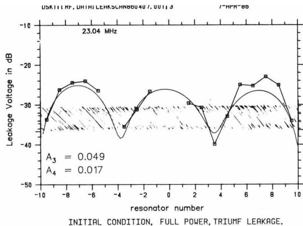
Fig. 5. Leakage voltage measured (squares) and calculated. The hash-marked band shows the range of voltages for which multipactoring can occur.
