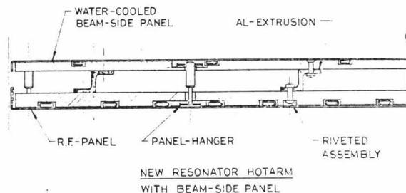
Fig. 7. Cross section of newly designed strongback.
