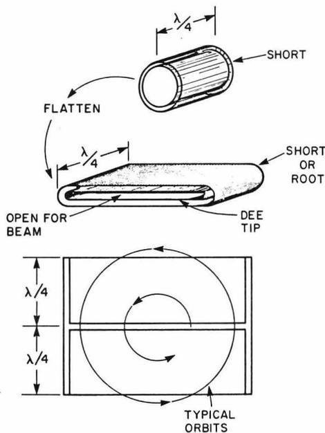
Fig. 1. Evolution of coaxial line into 2-dee resonator.
