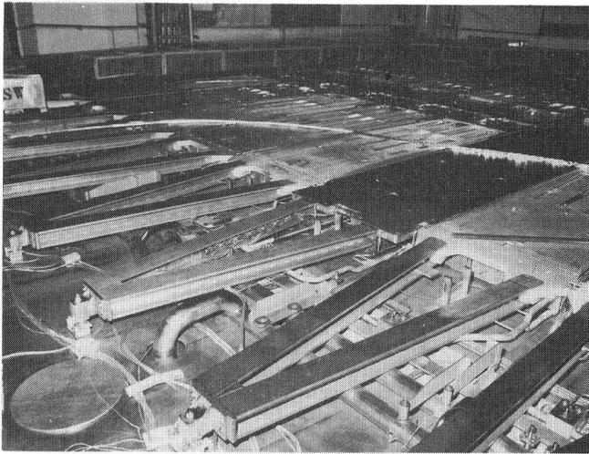
Fig. 3. View of lower segments in quadrant 3 with tank lid raised. The first segment with the newly designed beam-side panel is in position 5.
