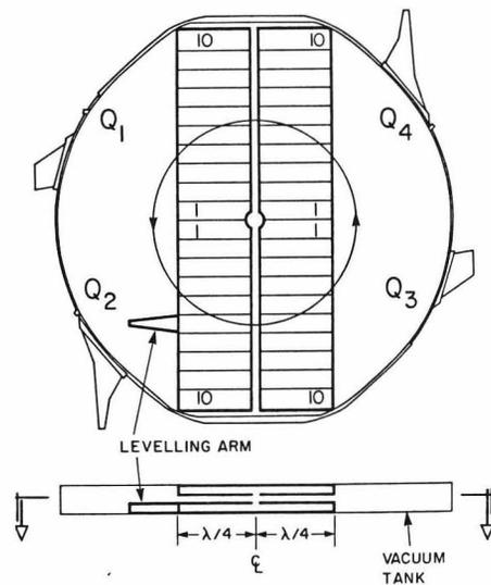
Fig. 2. Fitting of resonator in vacuum tank with support levelling arm for cantilevered strongback. Note segments are numbered 1-10, centre outward, in each of 4 quadrants.
