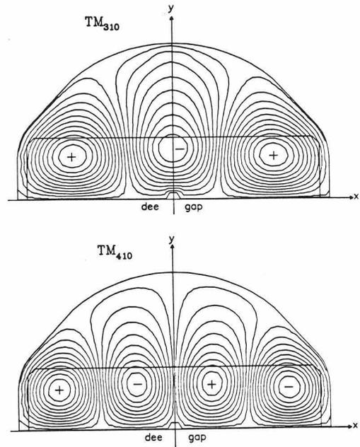
Fig. 4.  $TM_{310}$  and  $TM_{410}$  parasitic modes excited in beam gap.
