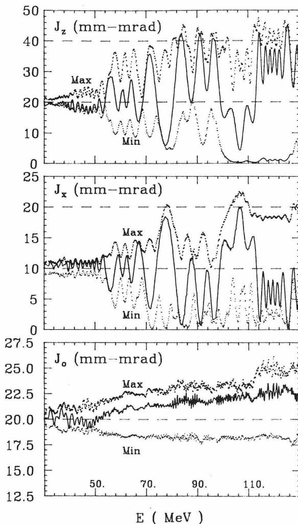
Fig. 4--Plots of  $J_z$ ,  $J_x$ , and  $J_0$  versus energy summarizing the data for eight orbits starting with  $J_z=20$  and  $J_x=10$  shown in Fig. 2. Solid curves are for one representative orbit, while dotted curves give maximum and minimum values for all eight orbits. Broken lines at  $J_z=40$  and  $J_x=20$  show theoretical limits. Here  $J_0$  is theoretically equal to 20 for all these orbits. See Eq. (1).
