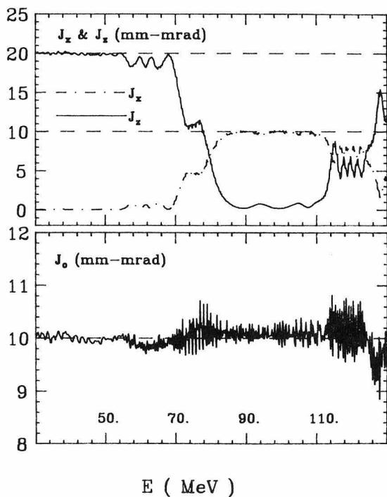
Fig. 3--Plots of  $J_z$ ,  $J_x$ , and  $J_0$  versus energy for one orbit that starts with  $J_z=20$  and  $J_x=0$ . The broken line at  $J_x=10$  is the theoretical maximum for  $J_x$ . Also,  $J_0$  is theoretically a constant. See Eq. (3) for units.
