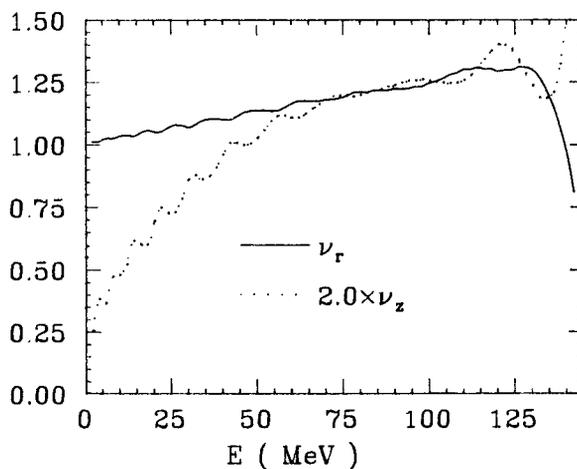
Fig. 1--Plot of  $\nu_r$  and  $2\nu_z$  versus energy showing that for this field, the operating point weaves around and remains close to the  $\nu_r=2\nu_z$  coupling resonance over a wide range of energies.
