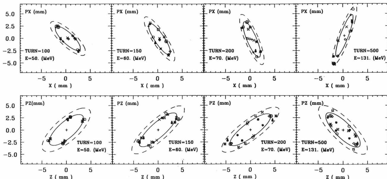
Fig. 5--Plots of  $p_x$  versus  $x$  (top) and  $p_z$  vs  $z$  (bottom) for 15 orbits on turns 100, 150, 200, and 500. These plots show evolution of points from an initially ordered state to a chaotic one. Solid eigenellipses have the same areas as the initial ones in Fig. 2, while broken eigenellipses represent theoretical upper limits for the growth in these areas.
