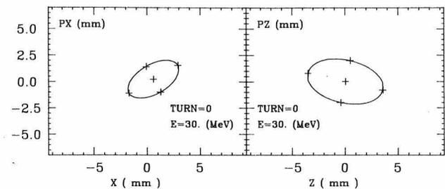
Fig. 2--Initial conditions for  $(x, p_x)$  and  $(z, p_z)$  on the two eigenellipses at 30 MeV corresponding to emittance values with  $J_x=10$  mm-mrad, and  $J_z=20$  mm-mrad. Note that the  $(x, p_x)$  eigenellipse is always centered on the "accelerated equilibrium orbit".
