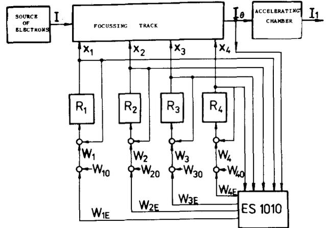
into the given value by the computer,  $x_i$  - adjustable parameters of the injector ( $I_f$ ,  $U_{tr}$ ,  $U_{r.c.}^{\oplus}$ ,  $U_{r.c.}^{\ominus}$ )  $I_k$  - the current of cathode source emission;  $I_{\theta}$  - beam current at the output of the rotary unit (optimized parameter).
