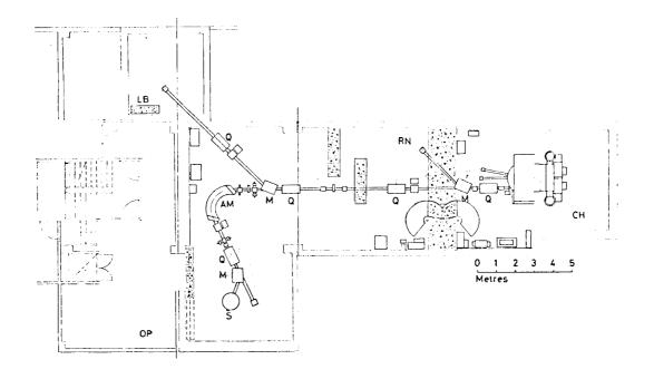
The layout of the compact cyclotron at Åbo Akademi(Finland): Q = quadropole lens, M = bending magnet, AM = analysing magnet, S = Scattering Chamber, LB = low background area, OP = controlroom, CH = cyclotron vault, RN = position for isotop production.
