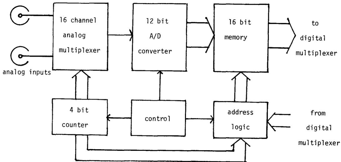
Figure 1. Block diagram of self-circulating analog multiplexer and A/D converter system
