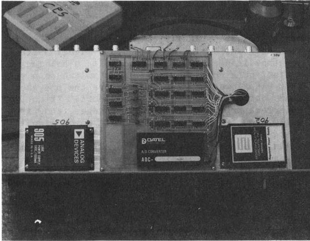
Figure 2. Self-circulating A/D system. Converter in center, flanked by power supplies and logic. Not shown (underneath) is analog multiplexer. Inputs are at rear.
