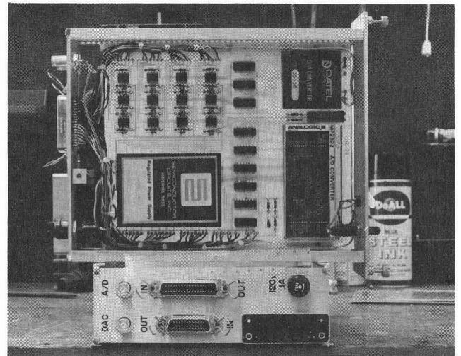
Figure 5. Floating power supply control module. Top view (upper module) shows all components. Rear view (lower module) shows digital and analog inputs and outputs, connector to power buss.
