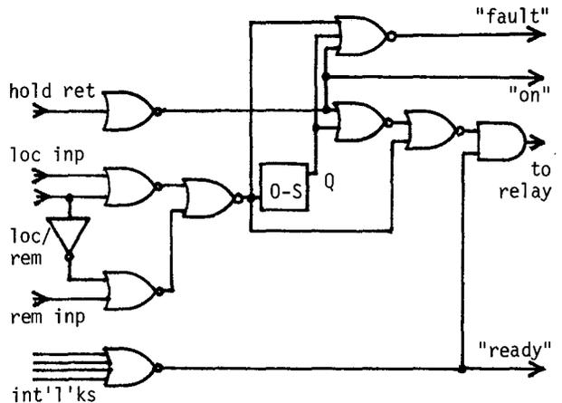
Figure 7. Logic diagram of ON/OFF circuit. Lamp and relay drivers omitted. "Low" is true for all inputs; "high" is true for outputs.
