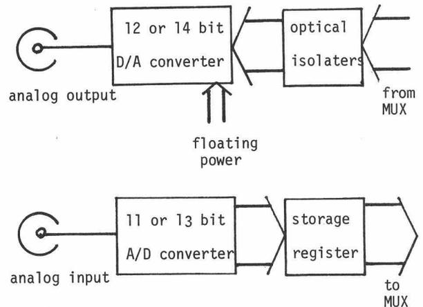
Figure 4. Block diagram of floating power supply control module
