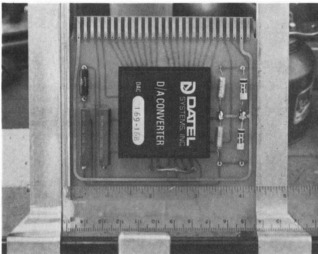
Figure 3. 16 bit D/A converter mounted on standard 52-pin card.
