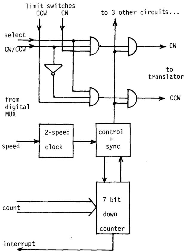
Figure 6. Simplified block diagram of stepping motor drive control circuitry.
