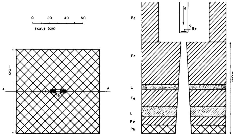
Fig. 2.- Front view and horizontal section (containing the beam axis) of the 19 x 4 cm neutron collimator (Fe = steel, L = lucite, Pb = lead)
