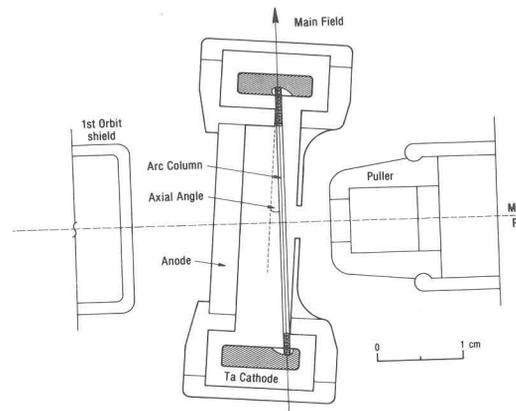
Fig. 1. The structure of the ion source head, axial rotation is about 5.5 degrees.
