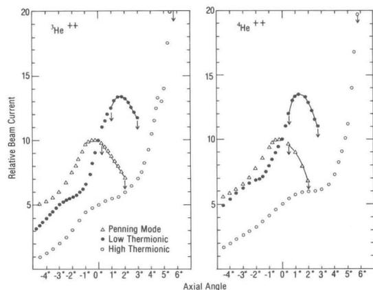
Fig. 4. Relative <sup>3</sup>He<sup>++</sup> and <sup>4</sup>He<sup>++</sup> beam current as a function of axial angle, relative scale applies to individual curve only.
