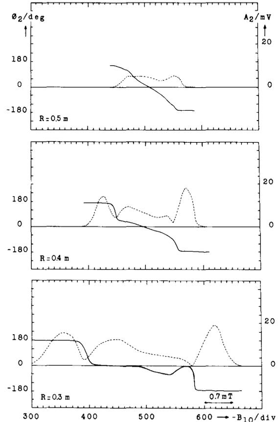
Fig. 3.1 The HF-phase (solid line) and the amplitude (dashed line) of the second harmonic of the probe signals at 30, 40 and 50 cm radius vs the magnetic induction of the outermost concentric correction coil B10. These curves are measured with the balanced mixers method at an internal beam current of  $1 \mu\text{A}$ .
