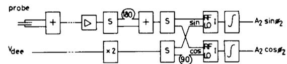
Fig. 2.2.1 A block schema of the phase measuring system using double balanced mixers. Signal splitters S are also used as adders +. In this experimental setup cables are used to perform phase shifts of 180° and 90°.
