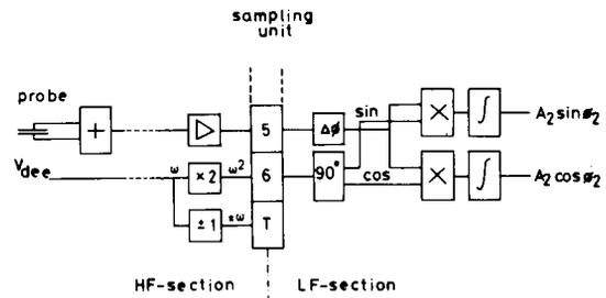
Fig. 2.1.1 A simplified block schema of the HF-phase measuring equipment. The sampling units are used to transform the phase probe signals (channel 1...5) and the reference signal (channel 6) from ~40 MHz (second harmonic) down to 1 kHz.
