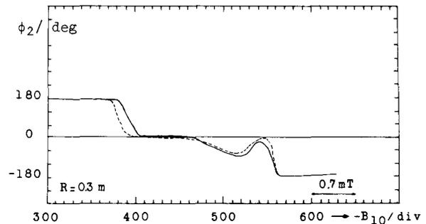
Fig. 3.2 The HF-phase of the second harmonic of the probe signal at 30 cm at an internal beam current of  $1 \mu\text{A}$  (dashed line) and  $30$  nA (solid line) measured with the balanced mixer system vs the magnetic induction of the correction coil B10.
