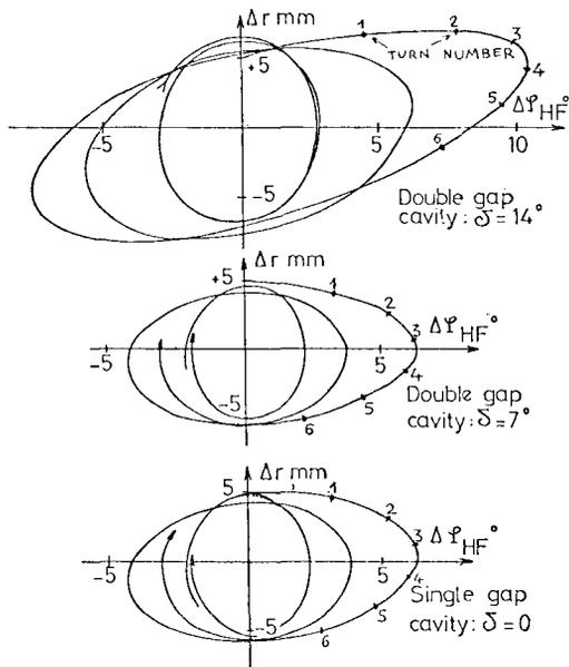
Fig 4:  $C_{12}^{+2}$  accelerated with  $h=16$   $k=5$
