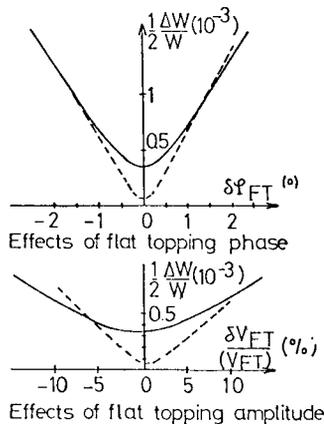
Fig1: Flat topping tolerances
