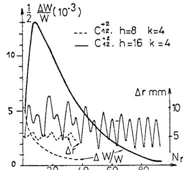
Fig 2 =  $\Delta W/W$  and  $\Delta r$  behaviour during the acceleration with 8<sup>th</sup> and 16<sup>th</sup> harmonics
