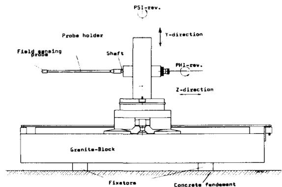
Fig. 1 The Measuring Machine
