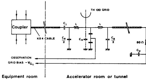
Fig.9: HF power amplifier matching filter .
