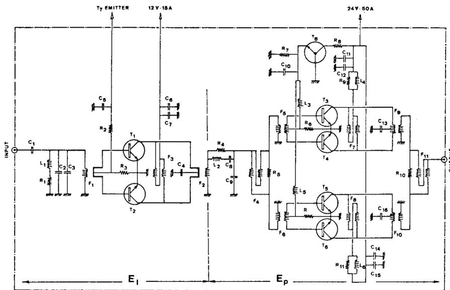
Fig. 1 : 100 W. solid-state wide-band amplifier module.
