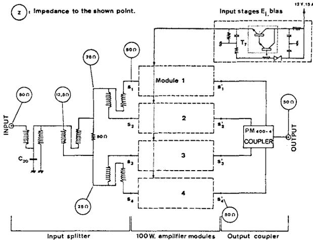
Fig. 2 : 400 w. solid-state modular amplifier and coupling circuits.
