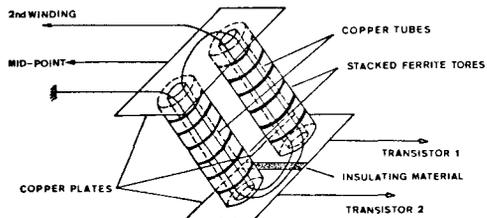
Fig. 3 : Impedance matching transformer with single turn .
