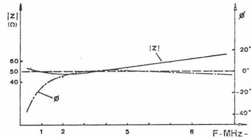
Fig.8: 100 w. modules input impedance.
