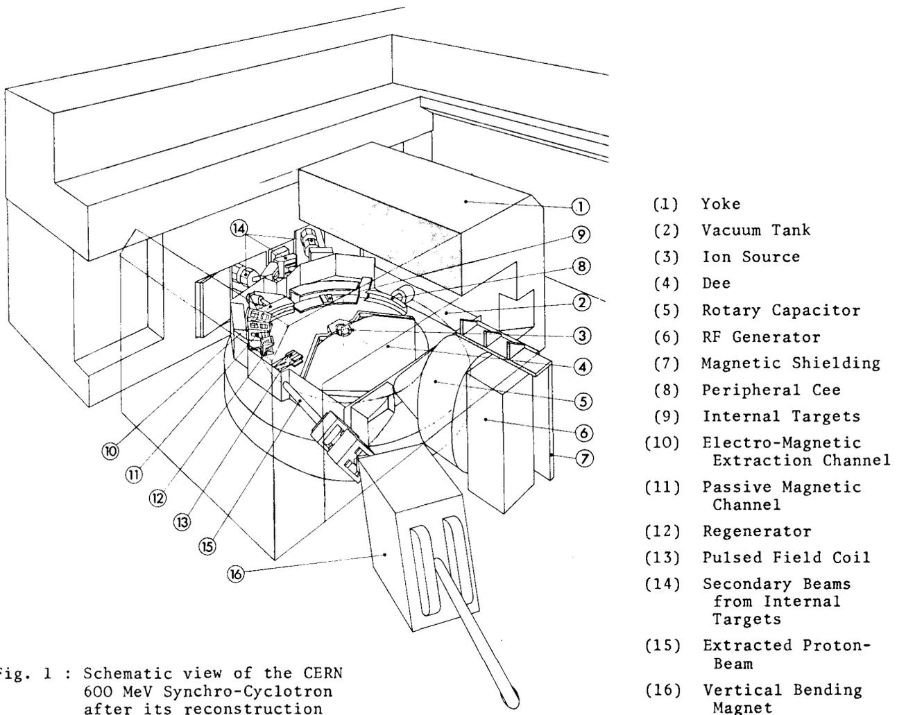
Fig. 1 : Schematic view of the CERN 600 MeV Synchro-Cyclotron after its reconstruction
