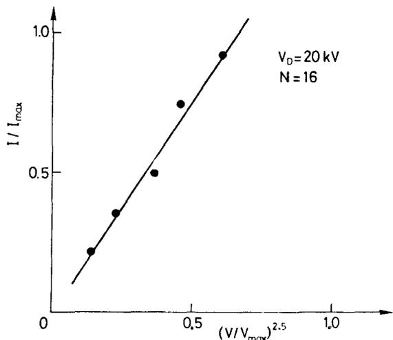
Fig. 6 : Internal beam as function of dee voltage
