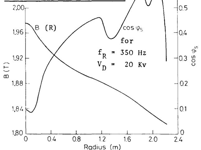
Fig. 3 : Magnetic field of SC2 and the cosine of the synchronous phase angle for  $f_R = 350$  Hz and  $V_D = 20$  kV as function of radius
