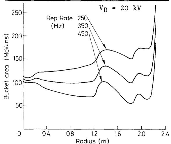
Fig. 4 : Bucket area as function of radius for  $V_D = 20$  kV and different pulse repetition rates
