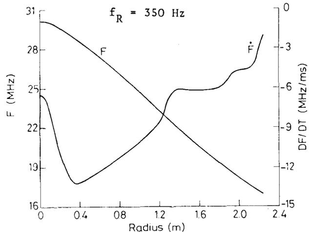
Fig. 2 : Resonant frequency and rate of frequency modulation at  $f_R = 350$  Hz as function of radius
