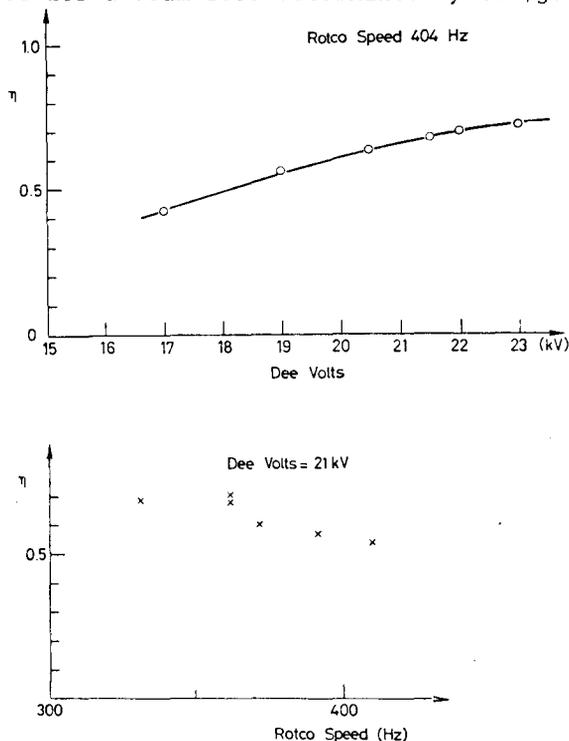
Fig. 7 : Extraction efficiency as function of dee-voltage and pulse repetition rate
