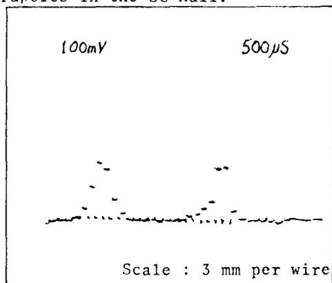
Fig. 8 : Horizontal and vertical profiles of the extracted proton beam, measured with a vacuum wire chamber
