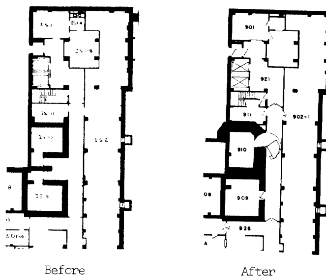
Fig. 1. Floor plans before and after installation of the cyclotron. The original facility had been designed for animal irradiation studies with ^{60}\text{Co} .
